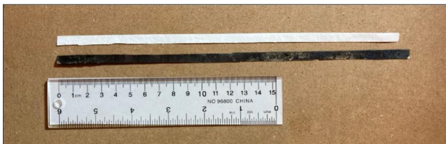
Figure 4 Strips of white (top) and blackened (bottom) TiO 2 on Glass Filter. Catalyst strips are 25-26 cm long and are shown here after synthesis and five washes with Milli-Q water.
