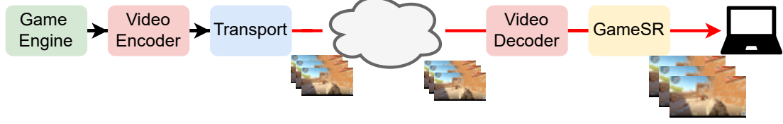
Figure 3.1: GameSR in cloud gaming: low-resolution streams are rendered at server-side and upscaled at client-side in real-time.
