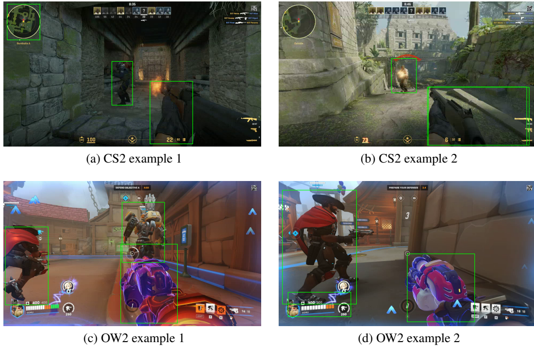
Figure 6.3: Client-side object detection as a post-decode plug-in. Annotated frames from CS2 and OW2 showing detector outputs computed after WebRTC decoding.
