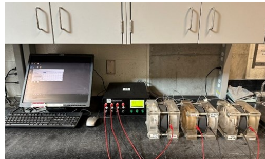
Figure 3.4. RCPT: (a) Schematic [13] and (b) Experiments in the laboratory.
