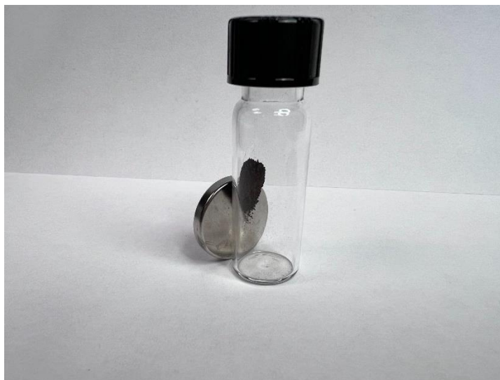
Figure S5.4.2. Fe 3 O 4 @TiO 2 after its synthesis next to a magnet to demonstrate its response to an external magnetic field.
