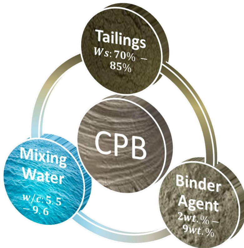
Figure 2.1 Components of cemented paste backfill (CPB)
