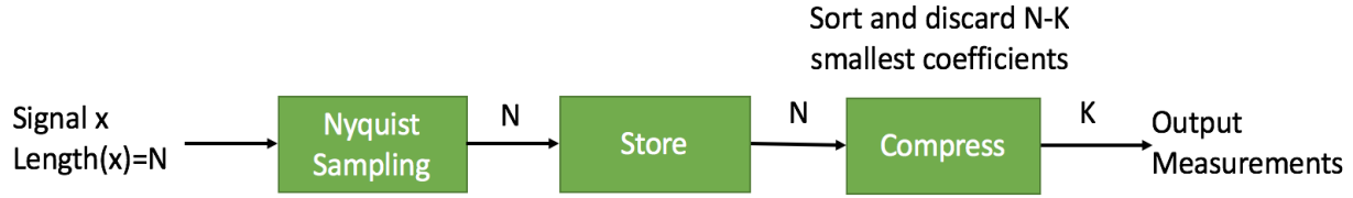
Figure 2 - Conventional transform coding scheme
