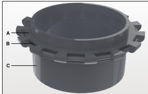
Figure 51: Valve assembly consists of (A) a top attachment, containing (B) a ratchet-like extrusion and an axis to support the winding leg systems, mounted to (C) an On-X 25 mm valve.
