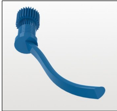
Figure 39: Bottom view of a single compression leg showing the ventricle-shape-conforming leg extension.
