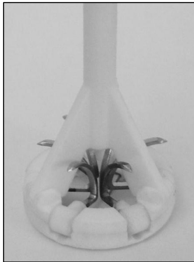
Figure 95: Prototype 1 of Concept 10: "Advanced hooks", un-deployed.
