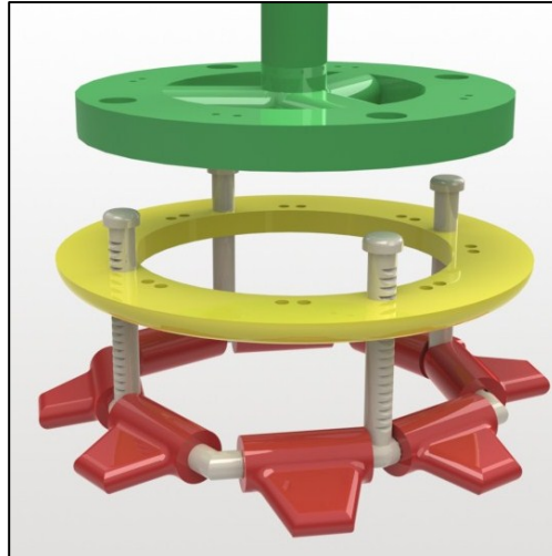
Figure 57: Deployed Concept 5 attachment base, with flaps extended and the holder partially removed.
