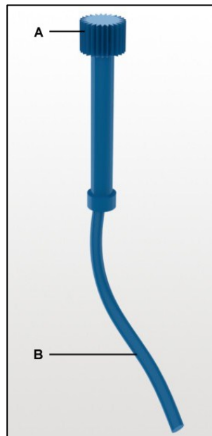
Figure 44: Compression leg system used for Concept 2, consisting of (A) gear mechanism, (B) leg extension.
