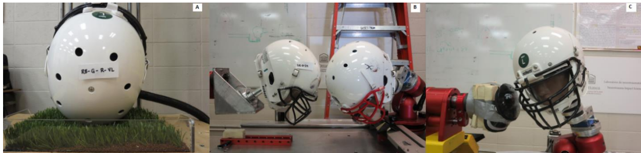
Figure 11. Reconstruction set-ups A) Falls B) Helmet-to-helmet collisions C) Shoulder-to-helmet collision.
