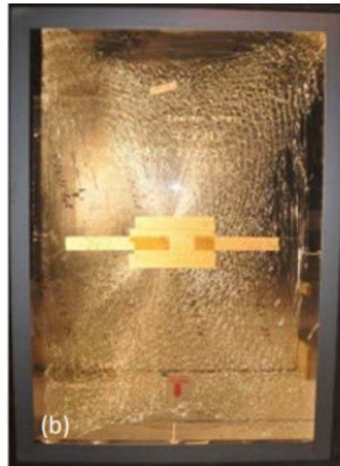
Figure 2.30: Window sample before test (left) and after test (right) (Lusk, 2011)
