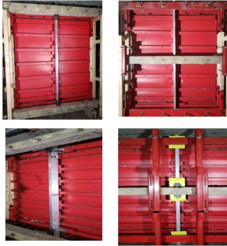
Figure 2.61: Testing mullions with different substrates
