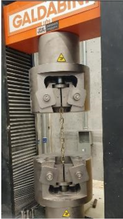
Figure 3.41: Tensile strength test for high strength chain
