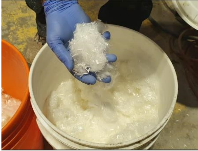
Figure 3.24: PVA fibers after air pressure application
