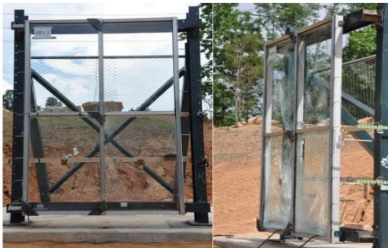
Figure 2.68: Specimen before (left) and after (right) the shot (Ralston et al. 2015)
