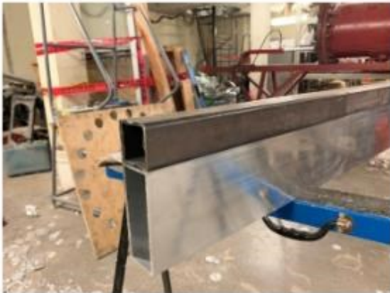
Figure 2.52: Tension flange hardened with HSS (left) and steel plats attached both sides (right) (Chavan, 2021)
