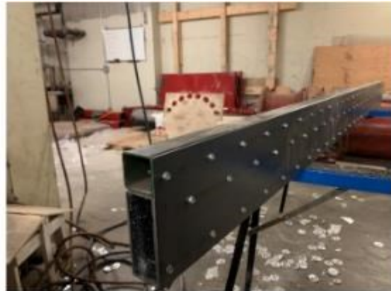
Figure 2.52: Tension flange hardened with HSS (left) and steel plats attached both sides (right) (Chavan, 2021)
