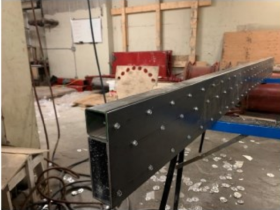
Figure 2.59: Mullion 3H with retrofitting (Chavan, 2021)
