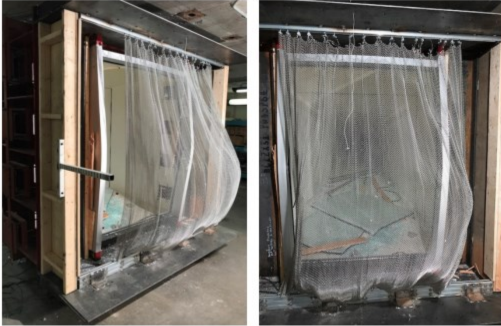
Figure 2.39: Curtain wall 1 after testing (Saatcioglu et al., 2017a)
