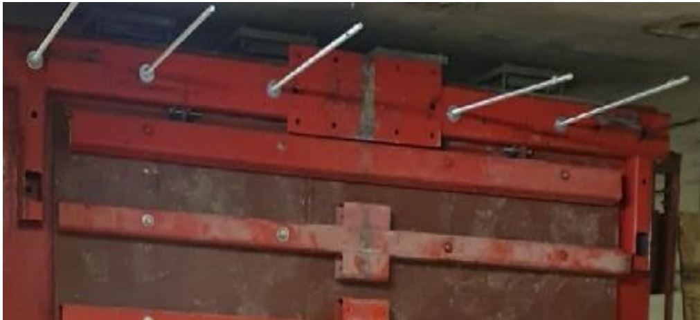
Figure 3.56: LTD attached to shock-tube opening by bolts
