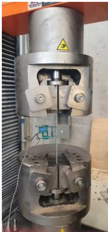
Figure 3.40: Tensile strength test for high strength wire
