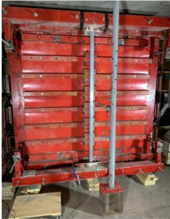
Figure 2.53: Load application devise generated the distributed load (Chavan, 2021)
