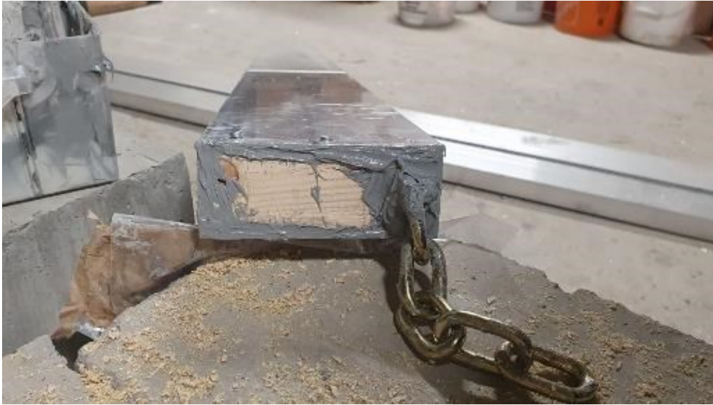
Figure 3.10: Epoxy paste for gap sealing
