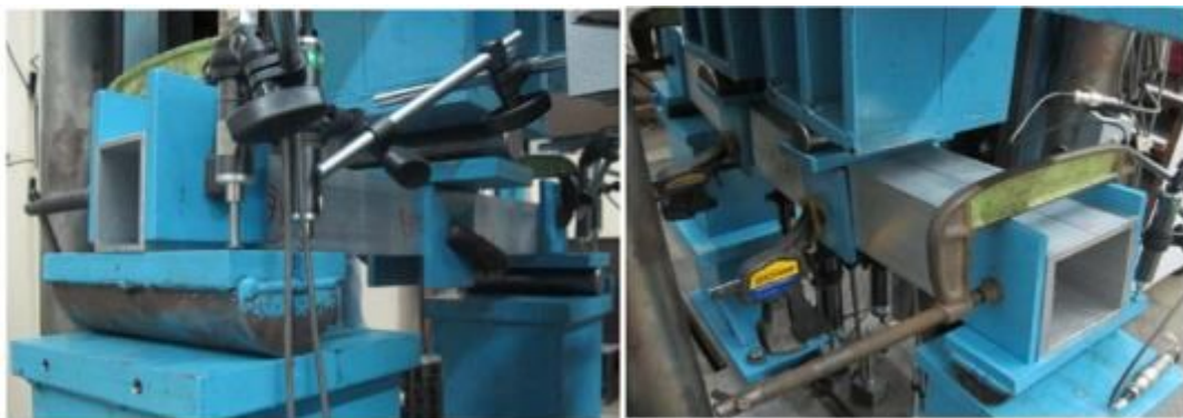
Figure 2.5: Experimental set up for three-point bending tests (left) and four-point bending tests (Right) (Su et al., 2014)
