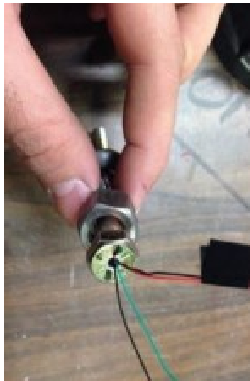
Figure 2.26: The instrumentation of anchors (Alameer, A., 2020)
