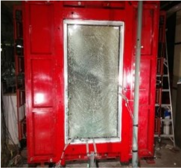
Figure 2.22: Wet glazing (Alameer, A., 2020)
