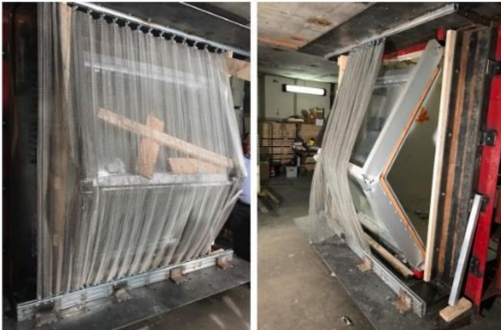
Figure 2.40: Curtain wall 2 with retrofitting after testing (Saatcioglu et al., 2017a)
