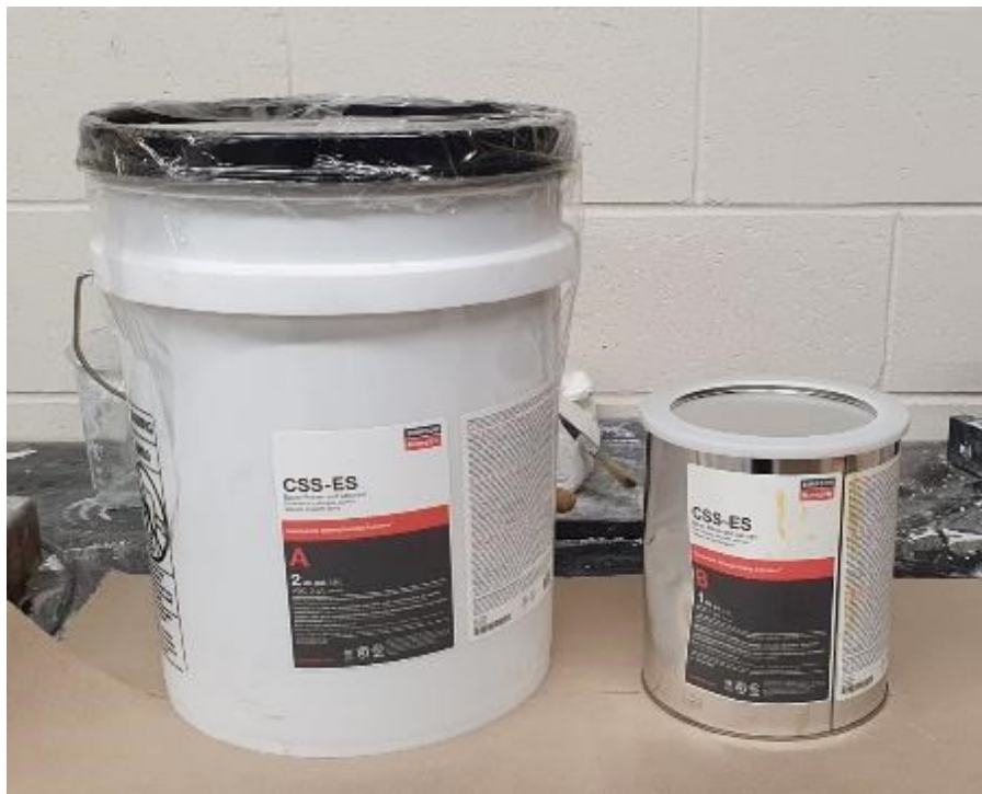
Figure 3.17: Two components (A and B) of epoxy mixture
