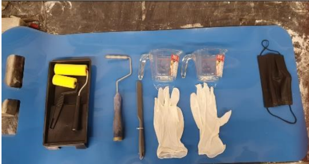
Figure 3.16: Tools used for epoxy application
