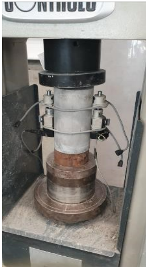
Figure 3.35: Compressive strength of HSM samples attached with LVDT
