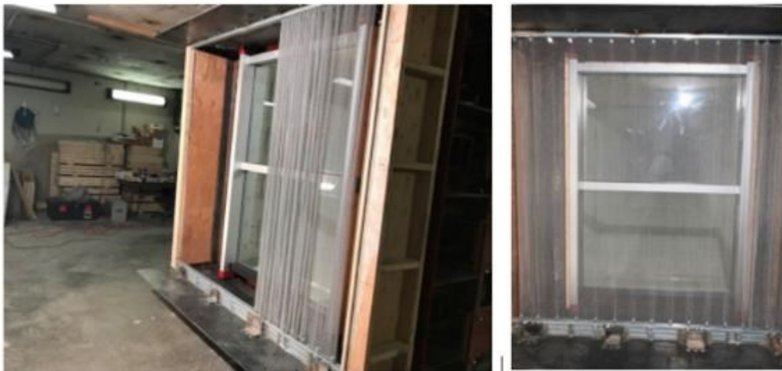
Figure 2.36: Curtain wall 1 prior testing (Saatcioglu et al., 2017a)
