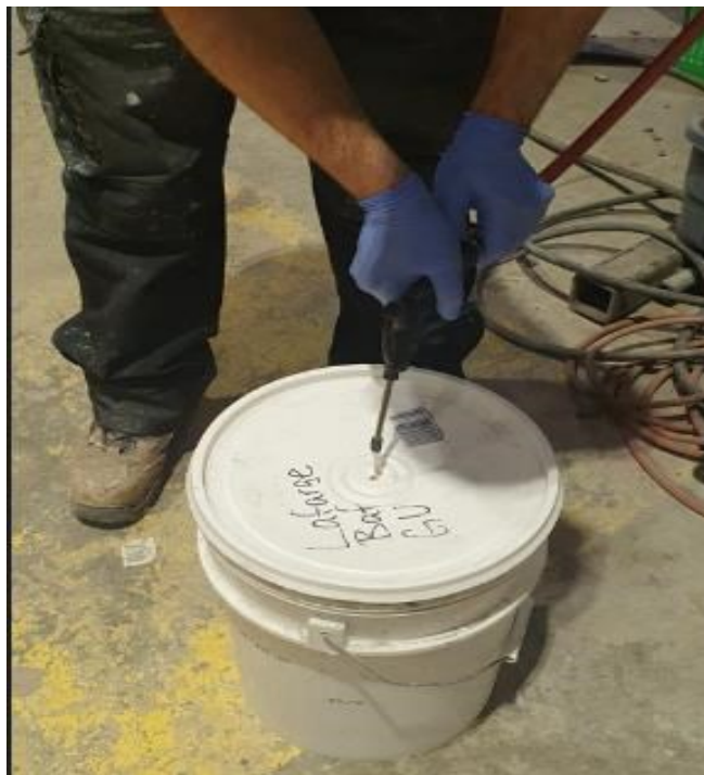
Figure 3.23: Pressure air application to disperse the fiber bundles
