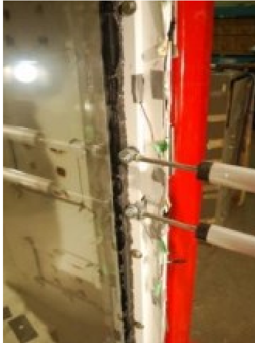
Figure 2.25: LVDT connection (Alameer, A., 2020)
