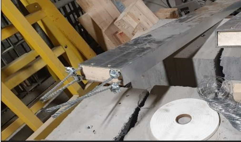
Figure 3.8: 1/4-inch Zinc-Plated Wire Rope Clip used to fix wires
