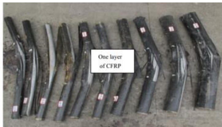
Figure 2.18: Concrete-filled aluminum alloy CHS tubes with one layer of CFRP (Chen et al., 2017)
