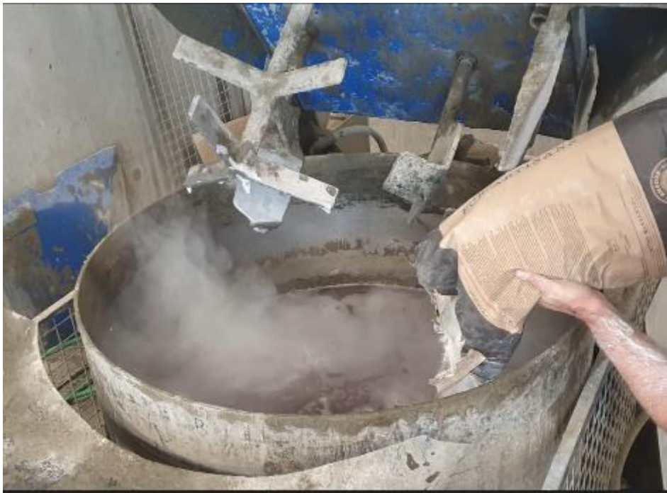
Figure 3.25: ECC powder addition to the water and superplasticizer mixture
