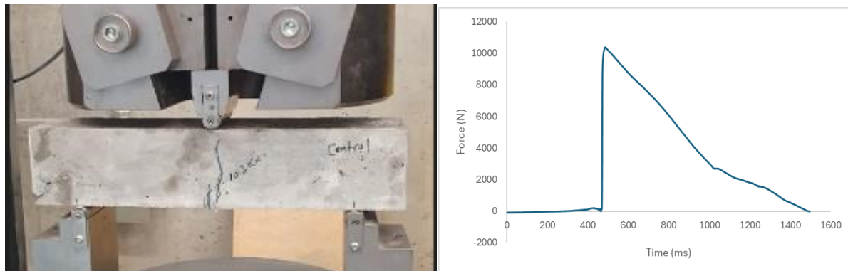
Figure 3.38: Flexural strength test for prism specimen without high strength wires
