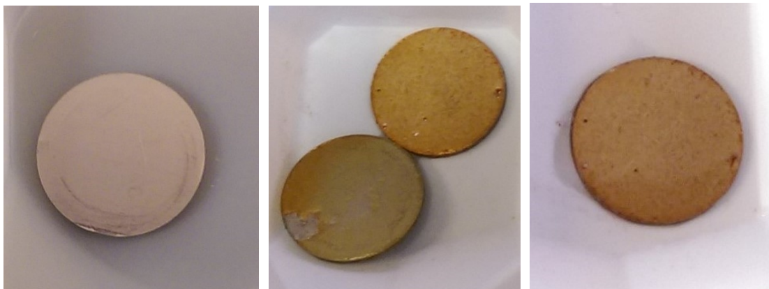
Figure 19: Photographic images of the titanium discs before treatment (left), after treatment (middle) and after 10 PBS washes (right) (Disc diameter=1.5cm).
