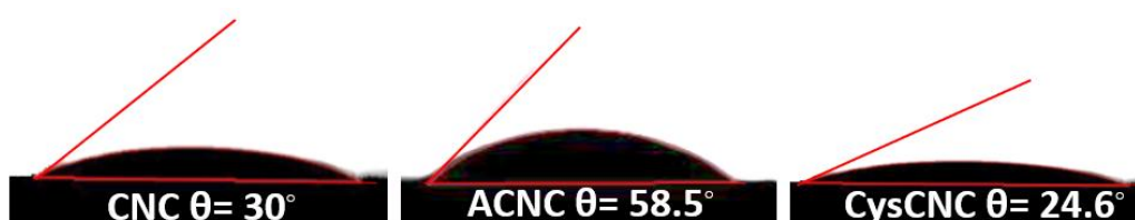
Figure 4.5: Water contact angle measurements of CNC, ACNC and CysCNC surfaces.
