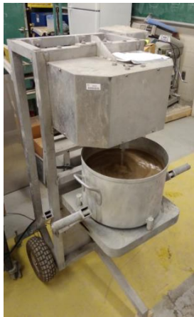
Figure 3.3. a) IBB rheometer and b) test programme used for analyzing the rheology cycle.
