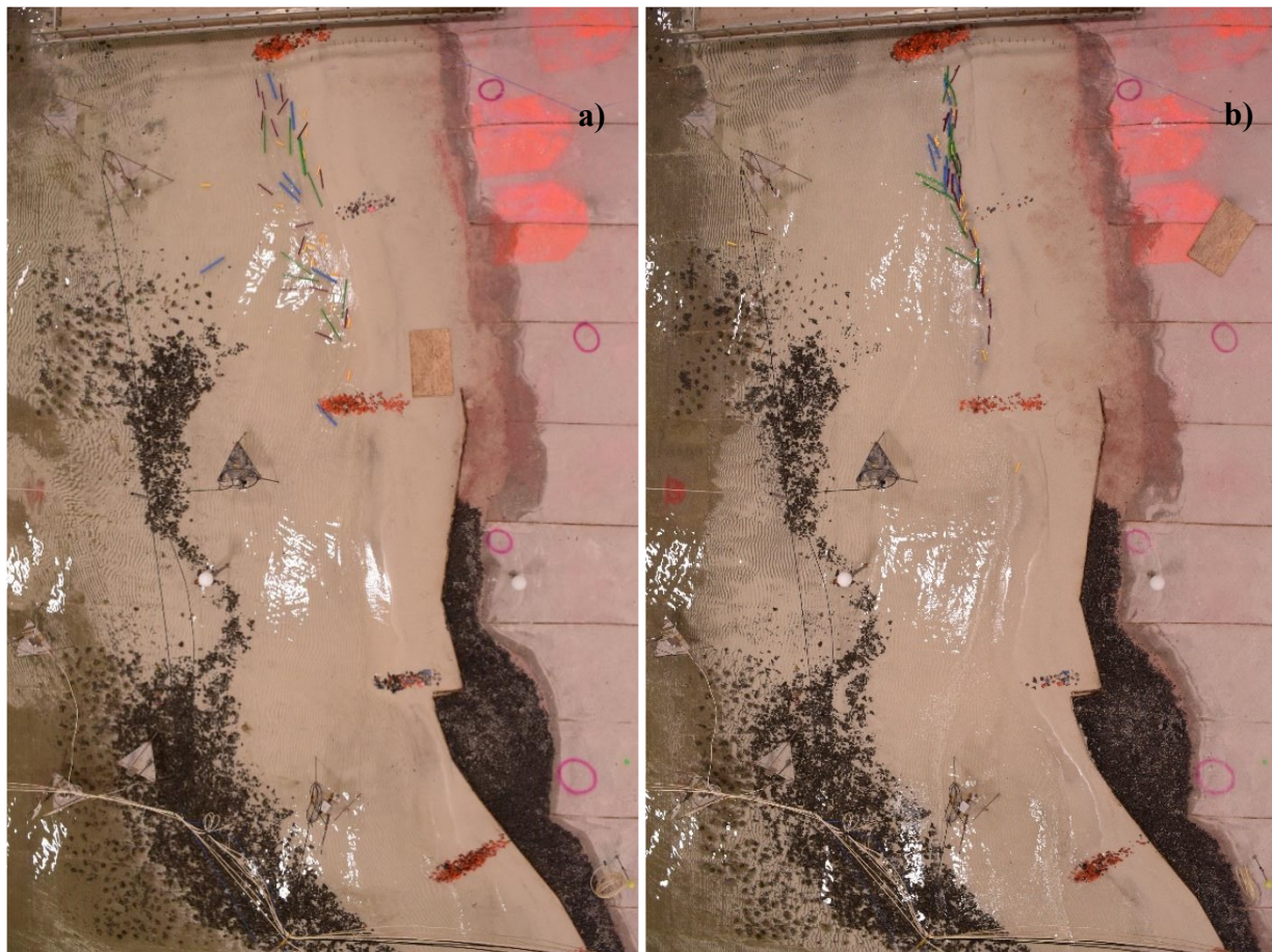
Figure 3-11. Instantaneous snapshots of driftwood in TS2 ( \eta = 0.35 m, H_{m0} = 0.65 s, and T_p = 8.0 s) at t = 400 s ( 12T_p ) after release, for a) smooth dowels, and b) rough tree branches.
