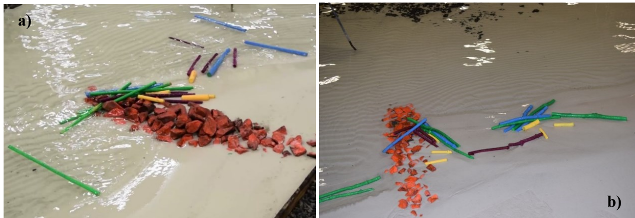
Figure 3-4. Model driftwood: a) dowels, and b) tree branches.
