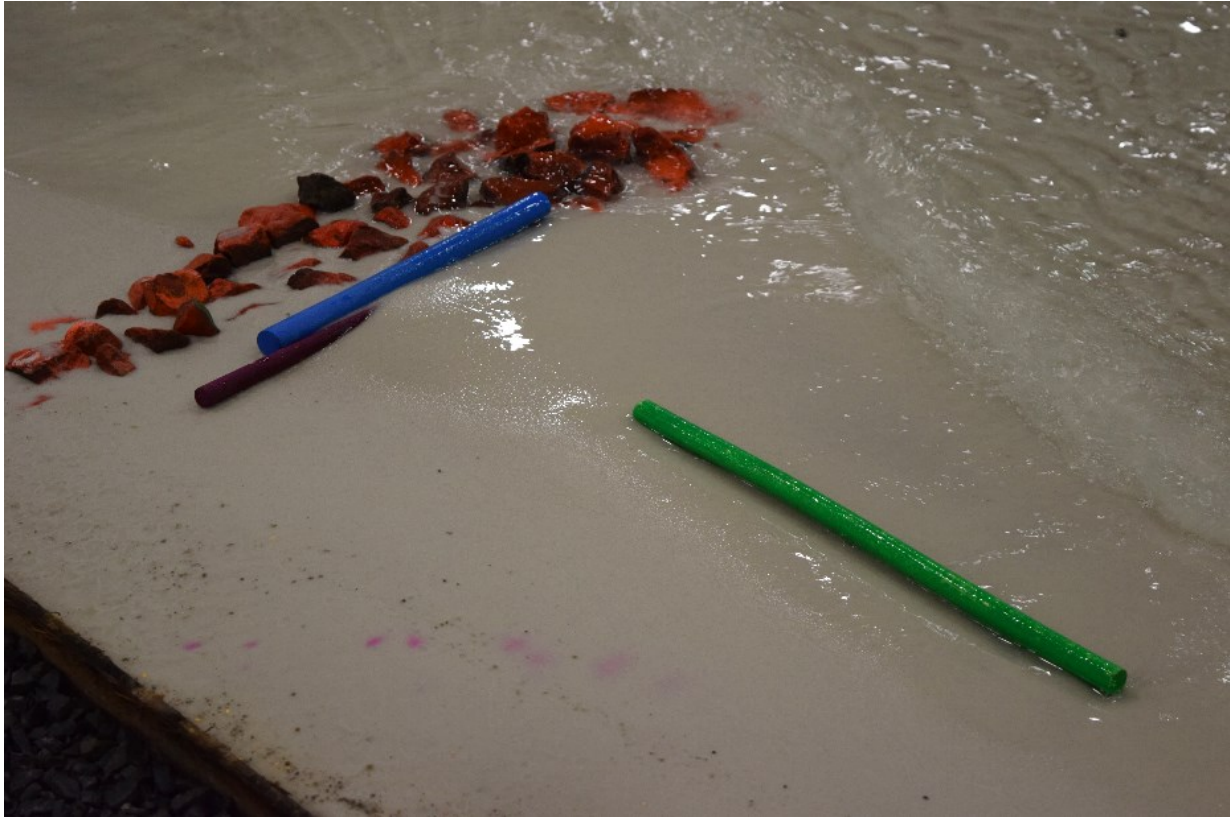
Figure 3-13. Driftwood partially buried by silica sand.
