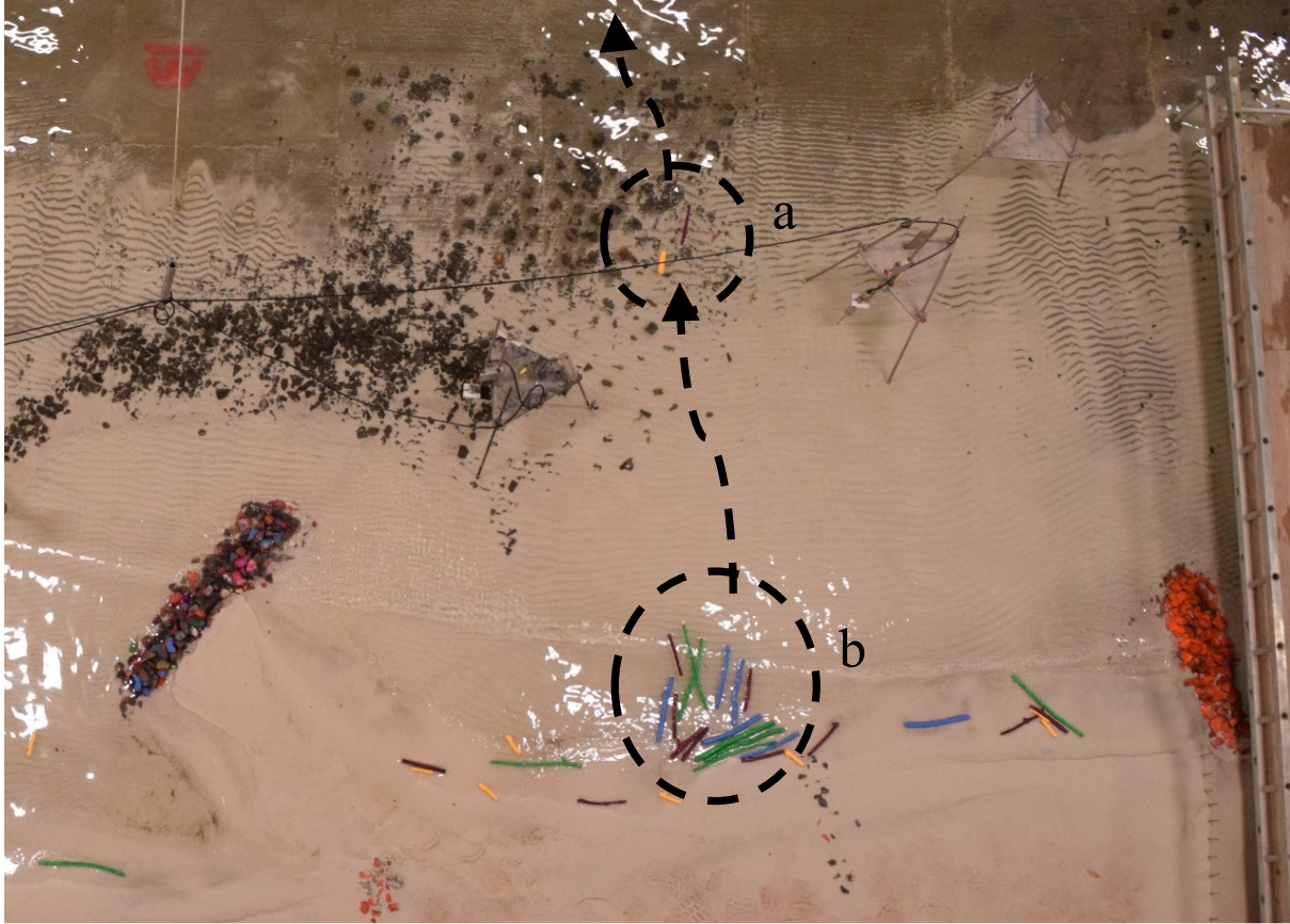
Figure 3-10. Snapshot showing effects of wave-driven circulation on driftwood transport
