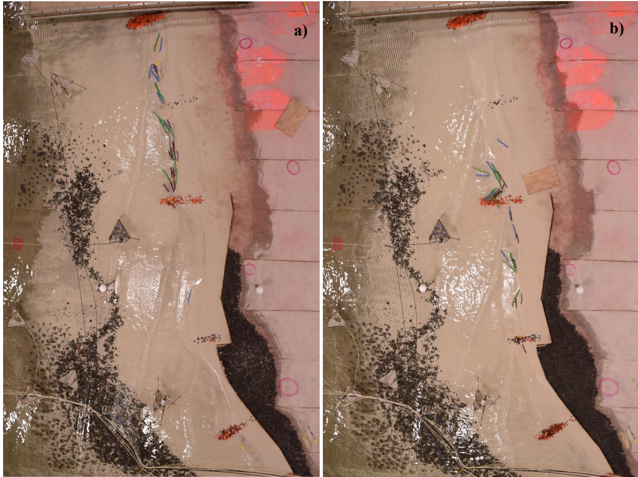
Figure 3-9. Snapshots (at t = 3286 s) of experiments a) TS2 and b) TS4, illustrating the effects of sea state on driftwood mobility.
