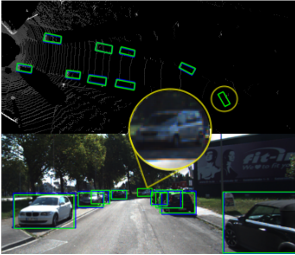
Figure 5.5: Sample from the KITTI dataset illustrating the capability of our network to accurately detect an object despite incorrect annotation. The green bounding box indicates true positive detection, while the blue bounding box represents ground truth.
