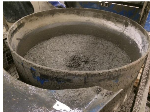
g) Concrete during mixing
