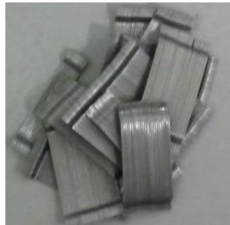
Figure 3-5 ZP 305 steel fibers
