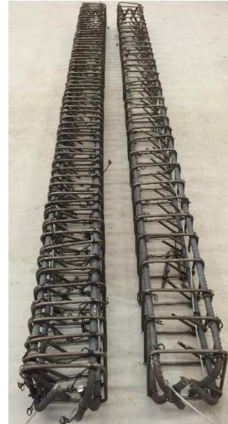
c) Seismic detailing vs. non-seismic detailing
