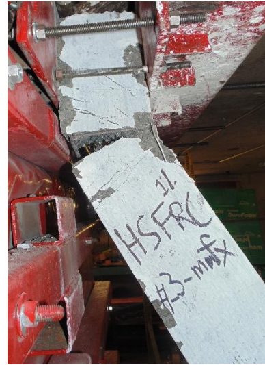
g) Top hinge and bar rupture at blast 4
