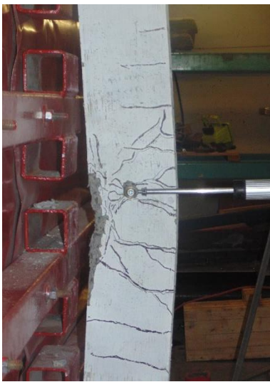
d) Mid-span at blast 3
