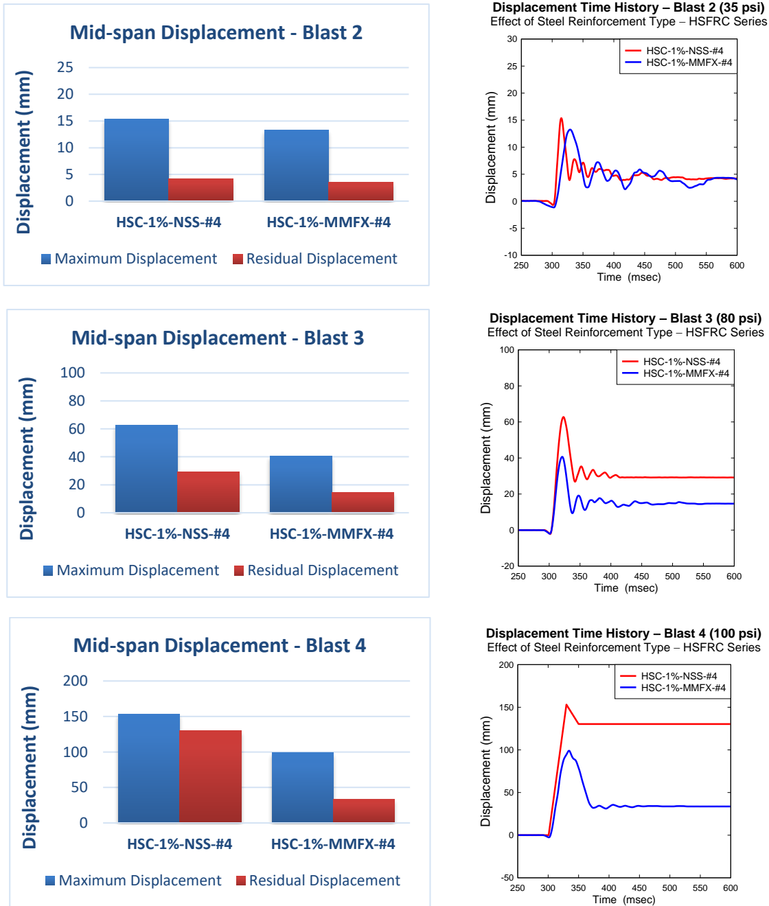
Figure 5-15 Effect of steel reinforcement type for HSC-1%-NSS-#4 vs. HSC-1%-MMFX-#4: Comparisons of mid-span displacements and displacement time histories for blasts 2-4
