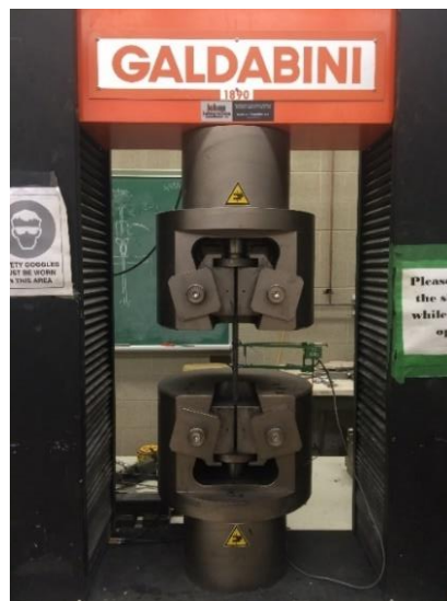
Figure 3-2 GALDABINI Universal Floor Standing Testing Machine used for steel coupons
