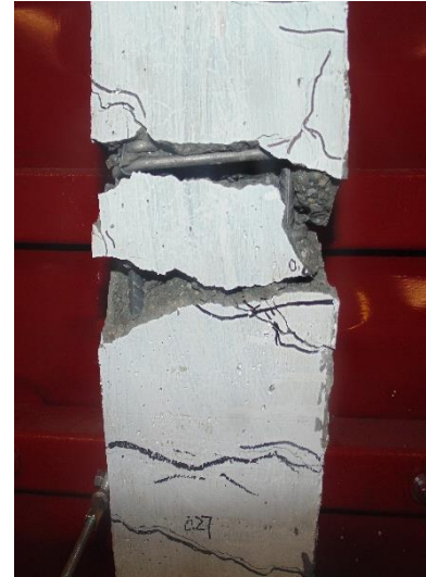
f) Major openings at blast 3
