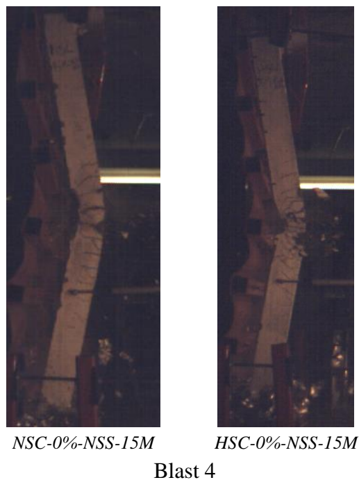
Figure 5-41 Effect of concrete strength on secondary fragmentation through high speed footage
