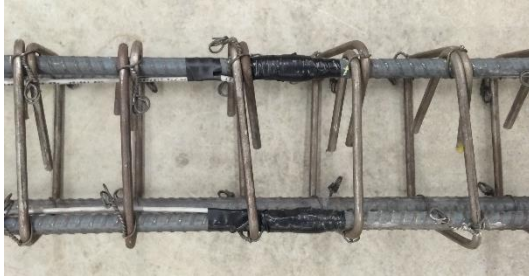
b) Strian gauges at the middle of the bars
