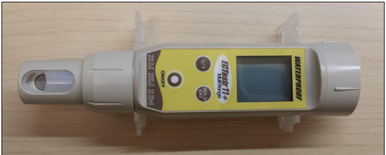
Figure 3-22: Cup-style sensor version of the solution conductivity-meter
