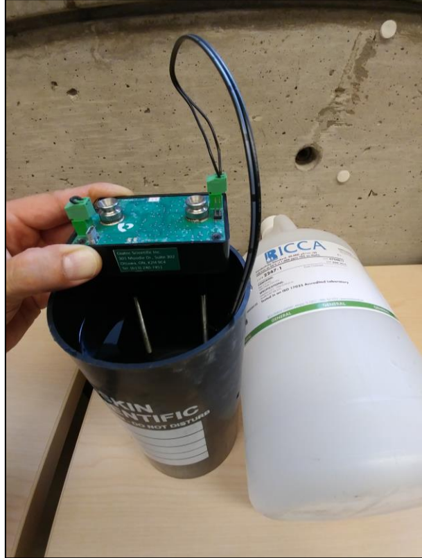
Figure 4-5: Measurement of the electrical properties of the standard conductivity solution
