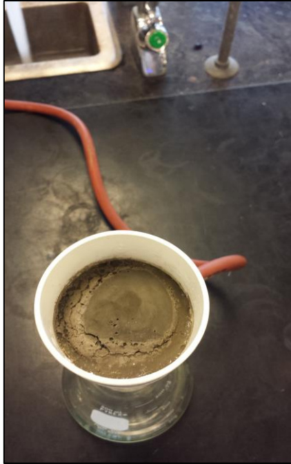
Figure 3-10: Extraction of pore solution from cement paste under direct vacuum suction
