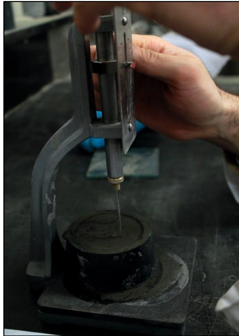
Figure 3-3: ASTM C191 test apparatus
