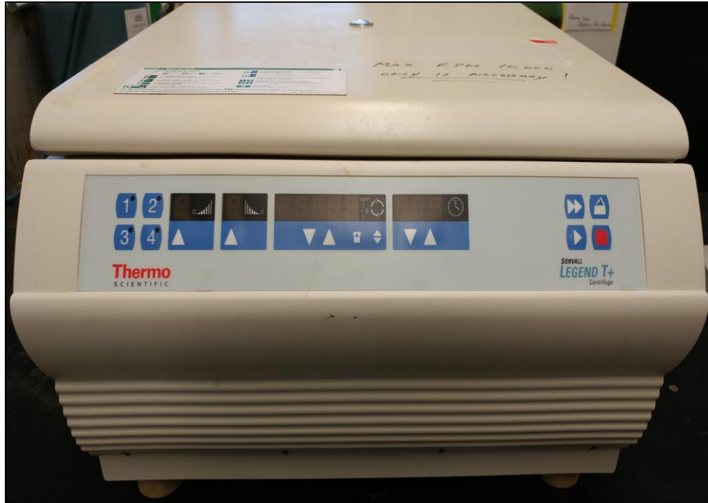
Figure 3-11: Legend T+ centrifuge for pore solution extraction from cement paste
