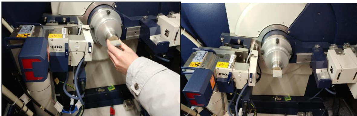
Figure 3-38: Cement sample placement in XRD machine
