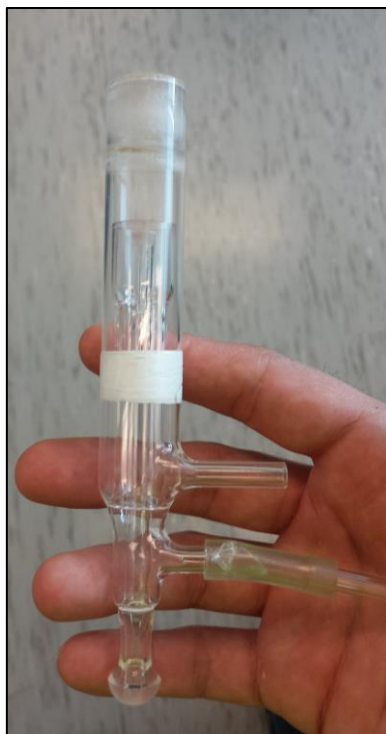
Figure 3-17: ICP-OES sample torch containing three concentric quartz glass tubes
