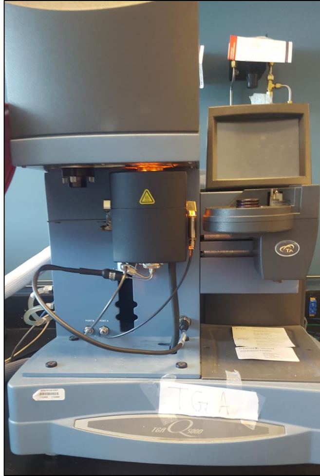
Figure 3-29: TGA universal V4.5A TA Instruments automated Q5000-IR
