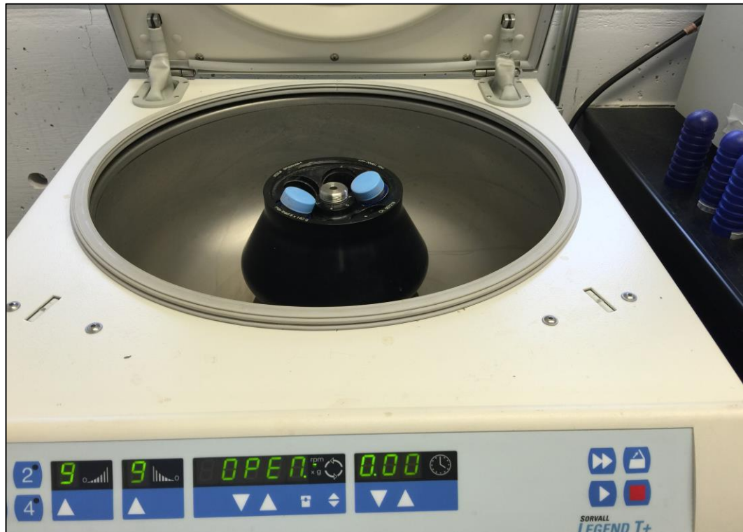
Figure 4-56: Sample set up in the centrifuge for pore solution extraction
