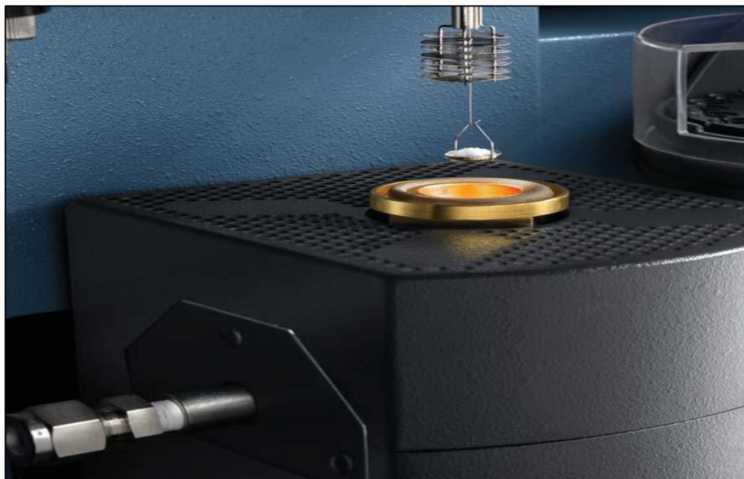
Figure 3-31: Sample placement in TGA (photo Courtesy of TA Instrument, Machine Manual)
