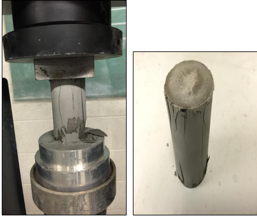
Figure 3-9: Compressive strength test sample and setup (left) and fracture pattern (right)
