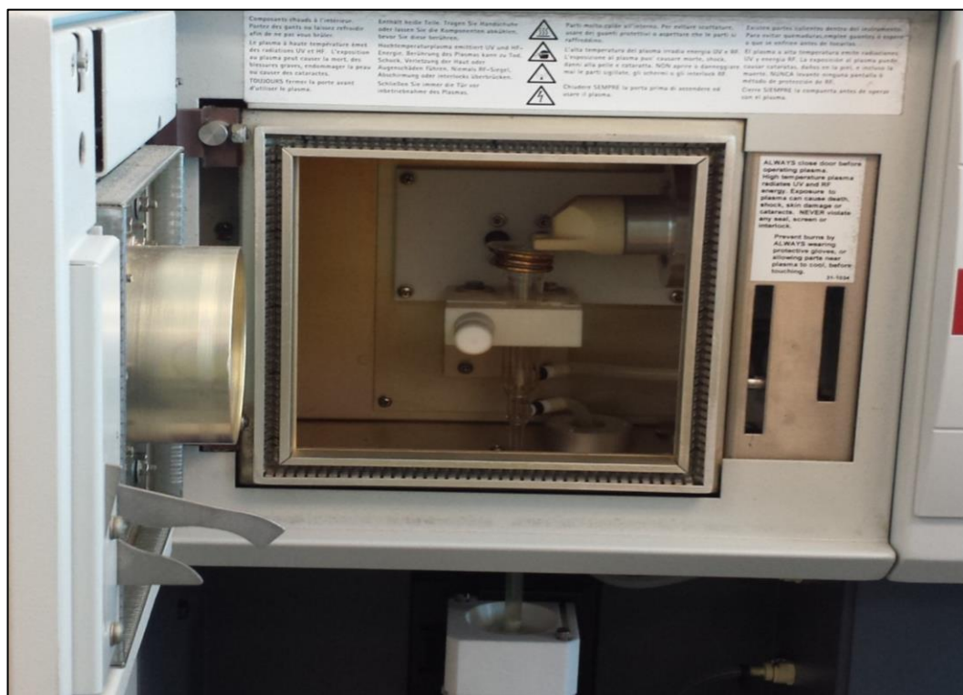
Figure 4-59: Set up of the concentric nebulizer in the ICP-OES
