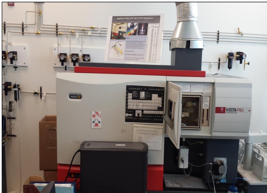
Figure 3-15: ICP-OES machine with CCD detector
