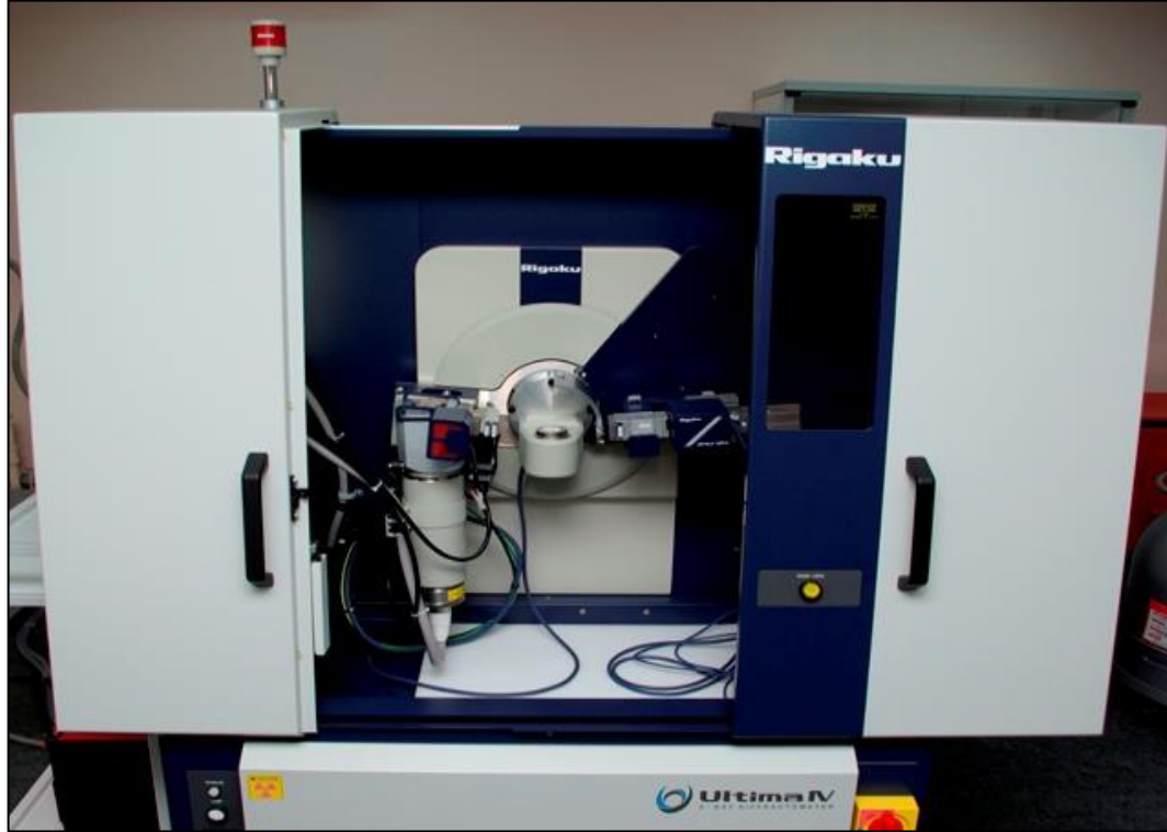
Figure 3-35: Rigaku Ultima IV powder diffractometer
