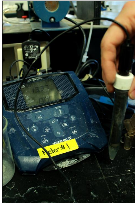
Figure 3-14: pH determination of extracted pore solution
