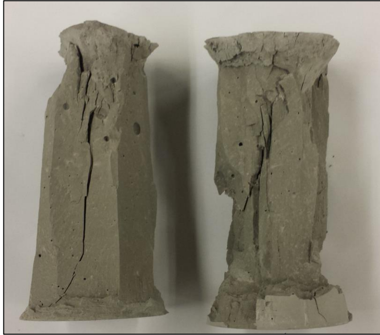
Figure 4-38: Comparison of fractured shapes resulting from compressive strength test (acceptable columnar fracture on right)
