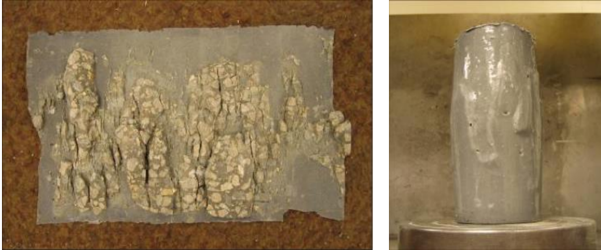
Figure 2.42 A concrete cylinder protected by polyurea
