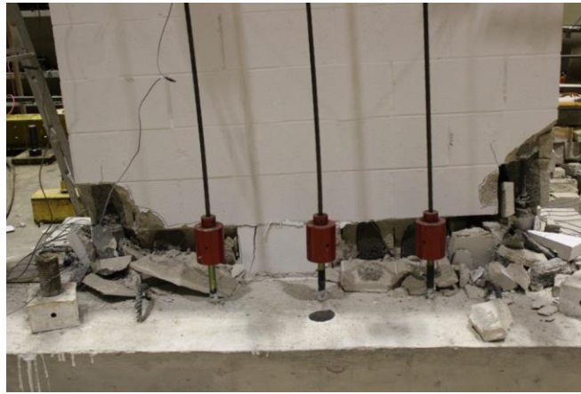
Figure 175.40 Wall 2 at 3.0% drift
