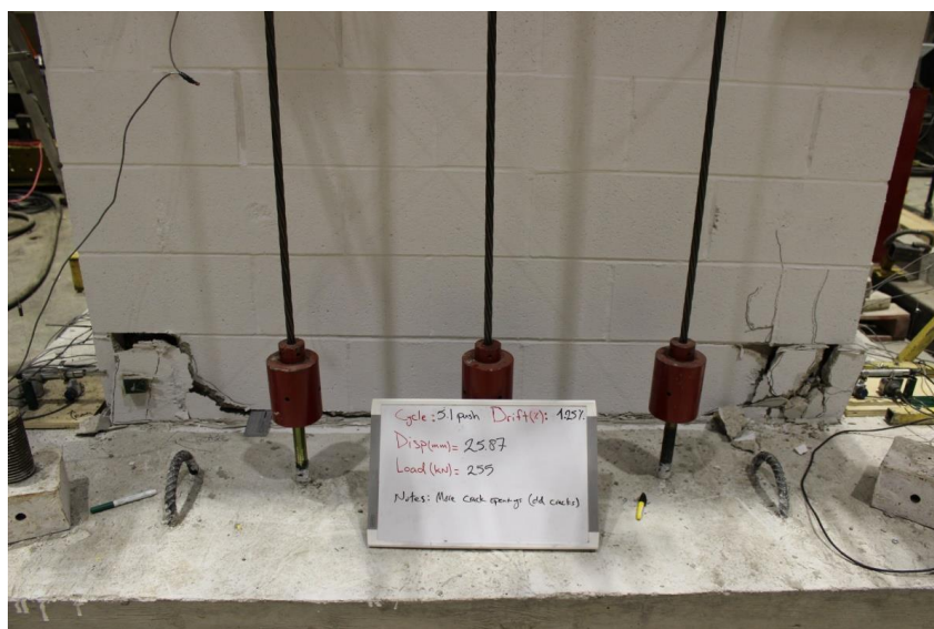
Figure 162.27 Wall 2 at -1.25% drift push
