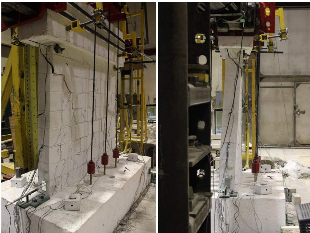
Figure 141.6 Twist of the wall at 0.5% drift
