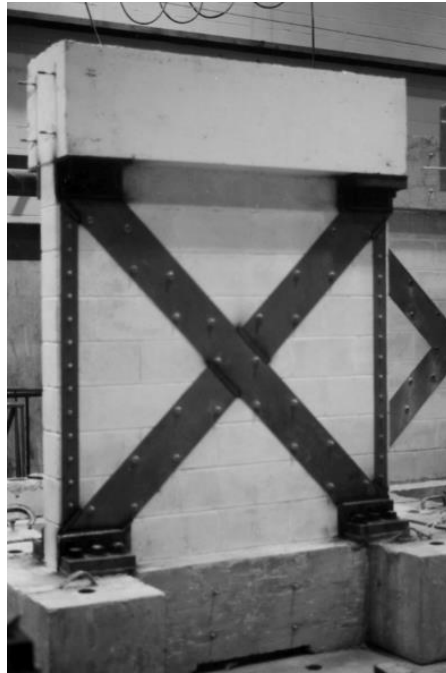
Figure 3.2 A masonry wall retrofitted by steel strips
