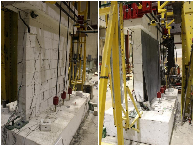
Figure 147.12 Damage of the wall at 1.25% drift ratio
