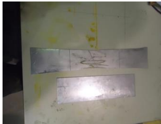
Figure 2.23 Elongation in stainless steel sheet (60%)
