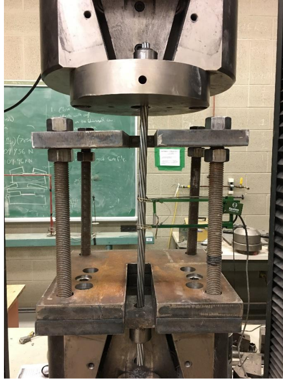
Figure 99.21 Coupon test setup for prestressing strand #15
