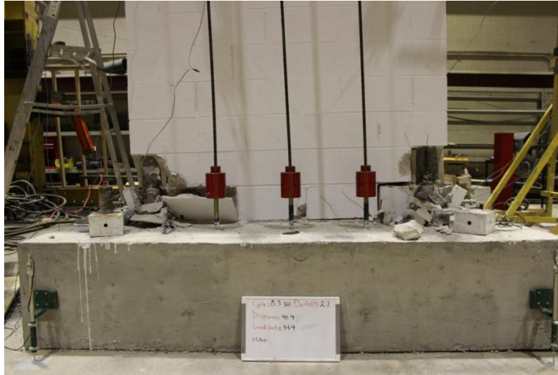
Figure 167.32 Wall 2 at -2.0% drift pull
