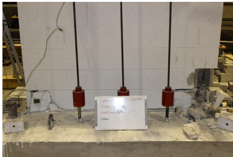
Figure 164.29 Wall 2 at 1.5% drift push
