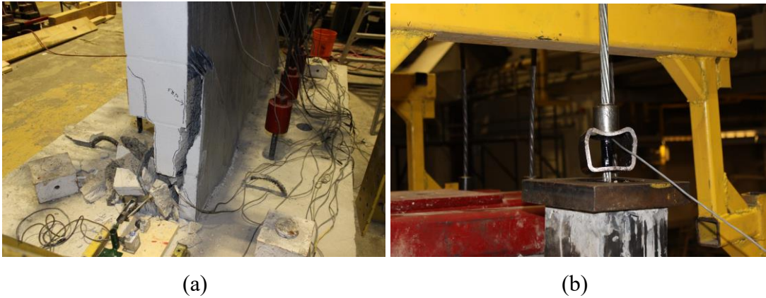
Figure 166.31 (a) FRP delamination and rupture at 1.75 % drift push, (b) HSS yielding agent at 1.75% drift pull (right)
