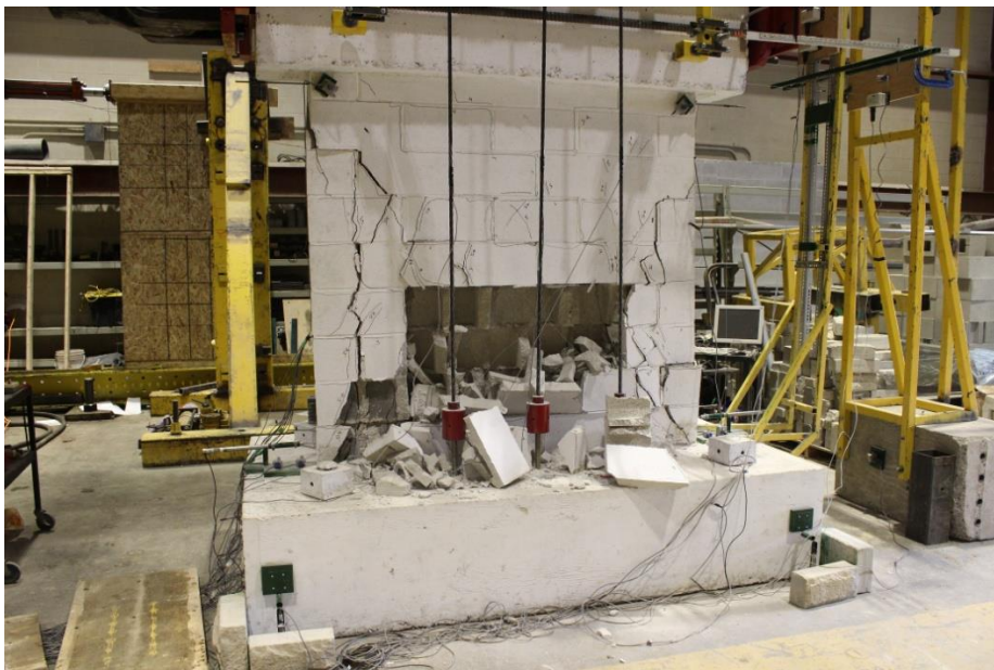
Figure 149.14 Final stage of the experiment for Wall 1
