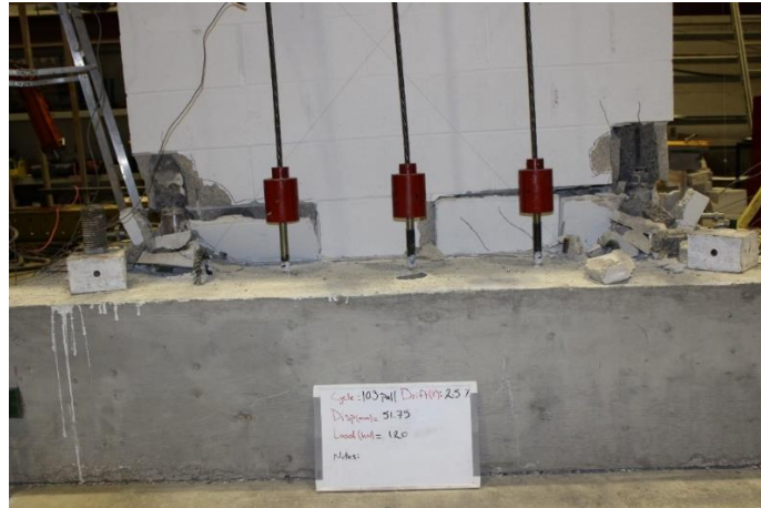
Figure 172.37 Wall 2 at -2.5% drift
