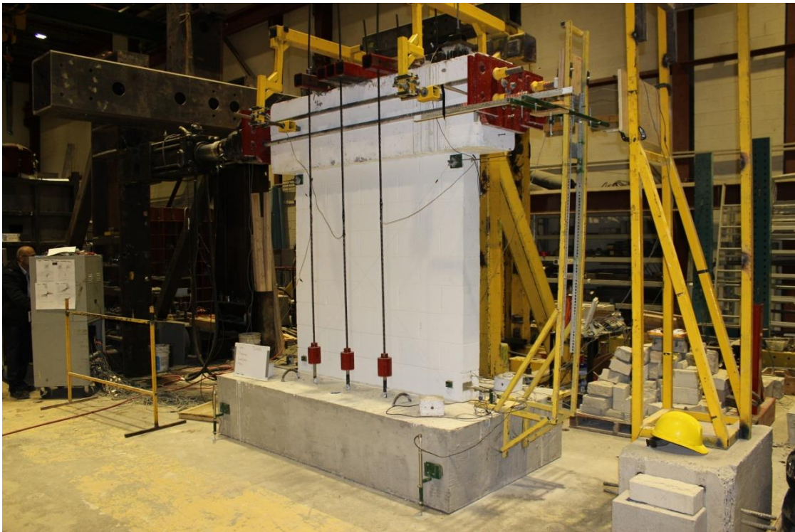
Figure 152.17 Retrofitted masonry wall 2 test setup
