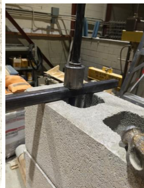
Figure 112.34 Post-tensioning cable secured at its place between to prestressing anchors
