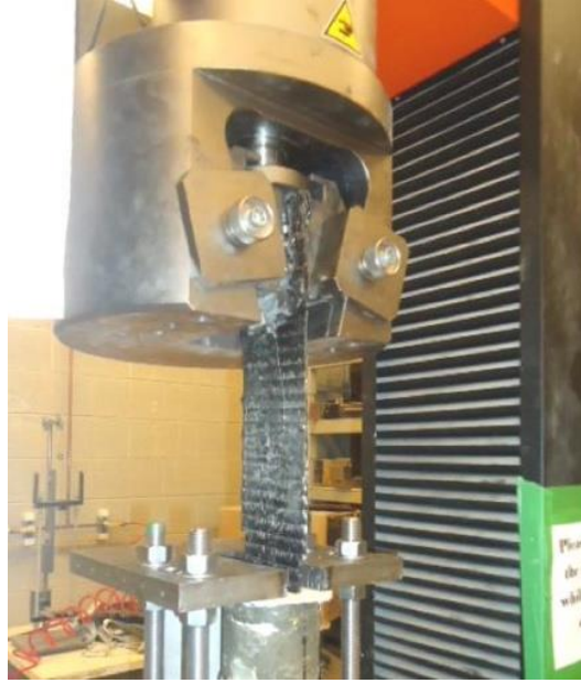
Figure 2.21 Pull-out test setup for FRP laminates
