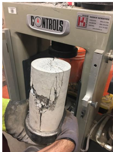
Figure 101.23 Failure of a concrete cylinder in compression
