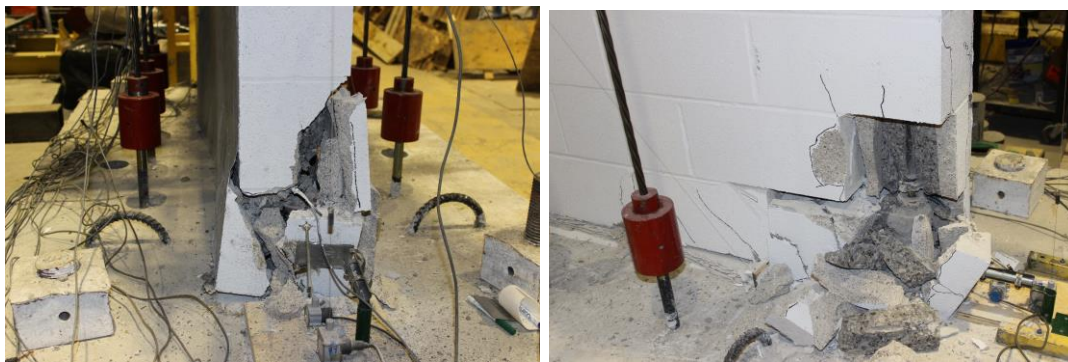
Figure 168.33 Toe crushing at west and east side, 2.0% drift ratio
