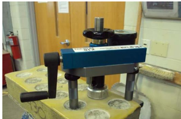
Figure 2.38 DYNA Z pull-off tester with digital manometer
