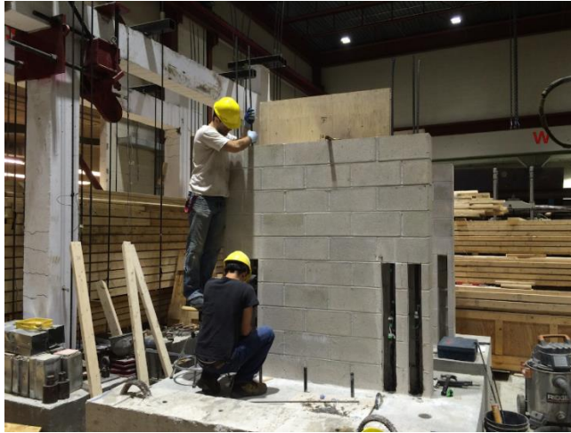
Figure 108.30 Installation of steel reinforcements inside pre-drilled holes by epoxy glue
