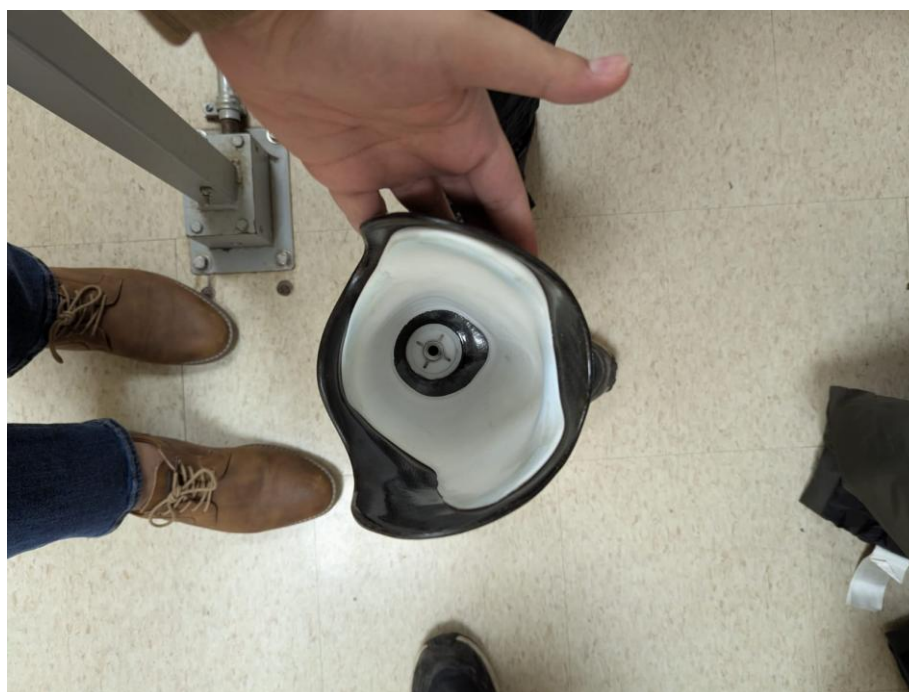
Figure 27: Socket insert with the distill opening centralised about the pin
