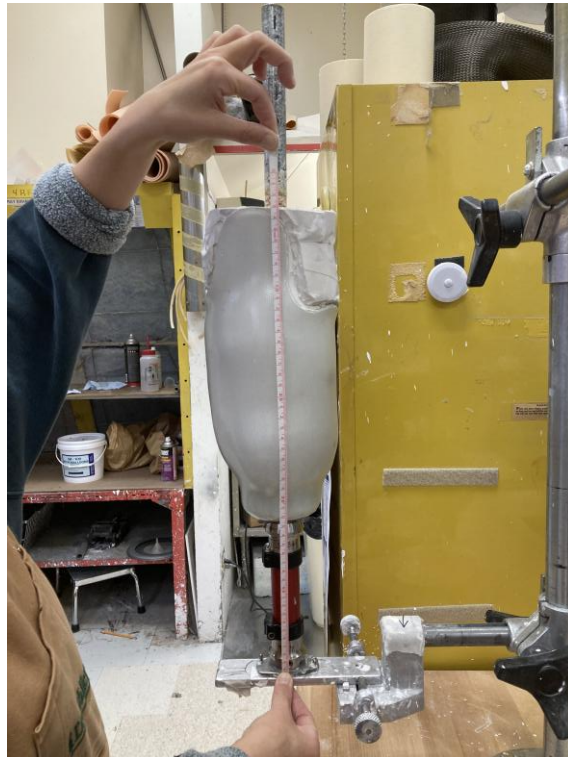
Figure 18: Socket-insert in the alignment jig. A tape measure identified the mandrel lock-pin location.
