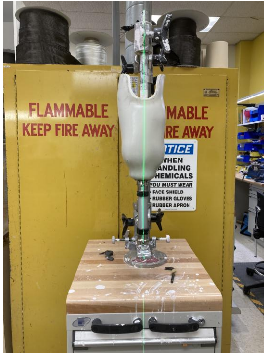
Figure 19: Socket-insert in the alignment jig. Laser is used to align the mandrel and the pylon.
