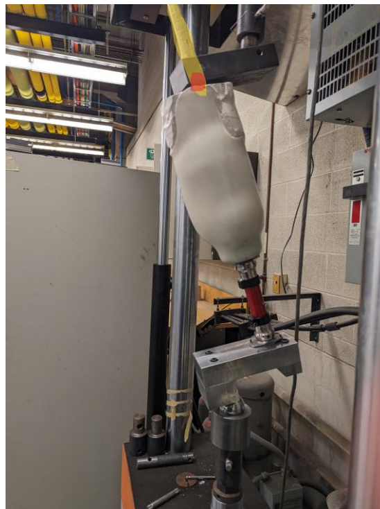
Figure 26: Socket-insert in toe loading configuration. Mandrel is highlighted in yellow. Bending location is highlighted in red
