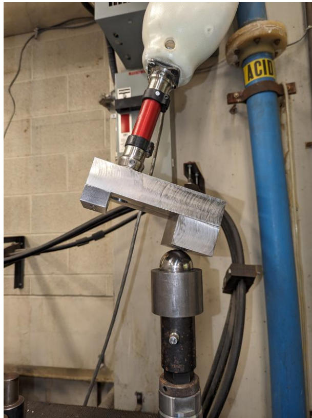
Figure 20: Bottom half of the testing setup in toe-loading configuration. Shown is the distal portion of the socket-insert, pylon, and bottom plate resting on the metal ball.
