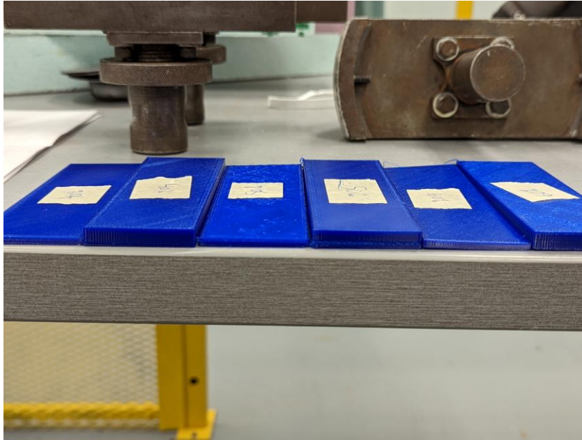
Figure 7: Six 3D-printed NCT blocks with 40%, 50% and 60% infill (3mm and 7mm thickness).
