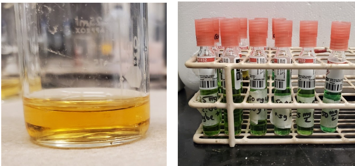
Fig. 3.4: Ammonia analysis methods; Ammonia solution after addition of Nessler reagent (left), HACH TNT-832 vials after the addition of ammonia solution (right).
