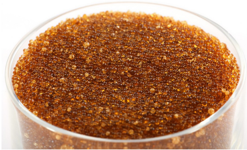
Fig. 2.4: Ion-exchange resin beads. (Ion Exchange in water treatment, 2022)
