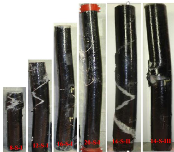
Figure 2.12 Failure modes of slender columns (Abdallah et al., 2018)
