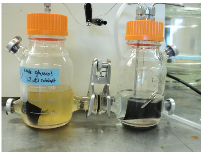
Figure 3.1: (Top) Schematic and (Bottom) photograph showing microbial fuel cell design
