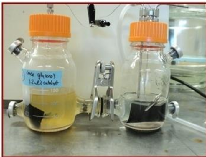
Figure 2.4: H-type fuel cell.
