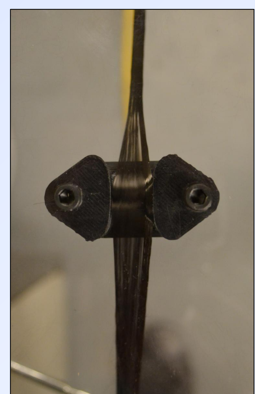
Figure 10 - Spreading the carbon fiber yarn
