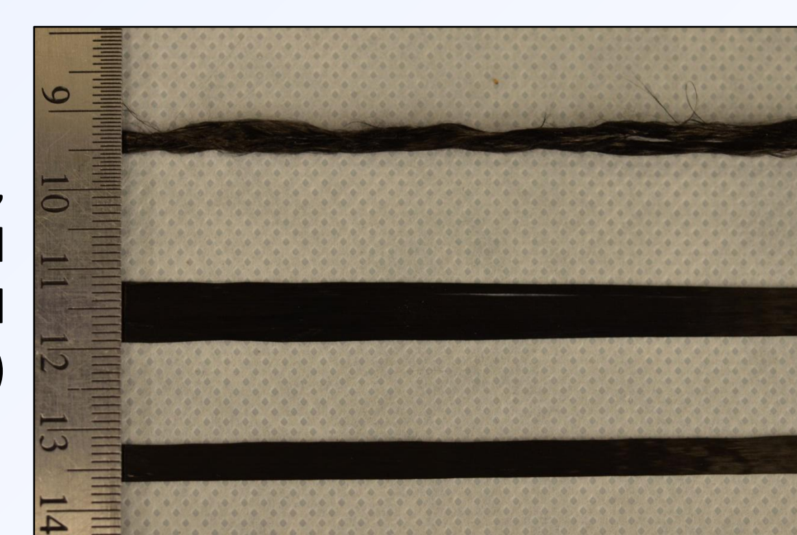
Figure 9 - Narrowed yarn (top), spread yarn (middle) and un-manipulated yarn (bottom)
