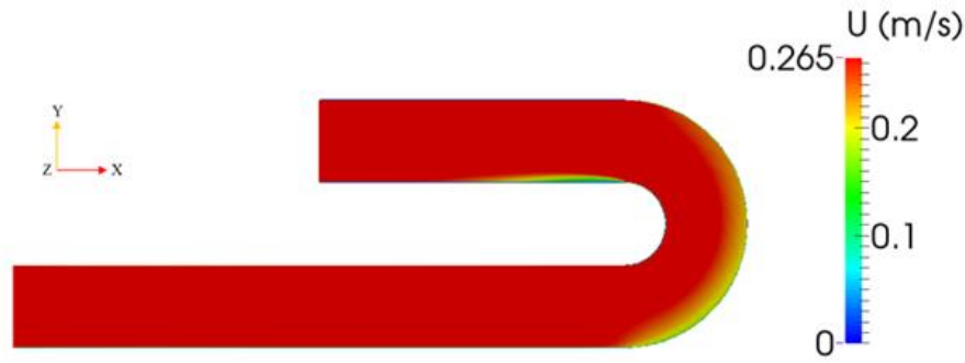
Figure 5.7: The distribution of water surface velocity (Realizable k-\epsilon )
