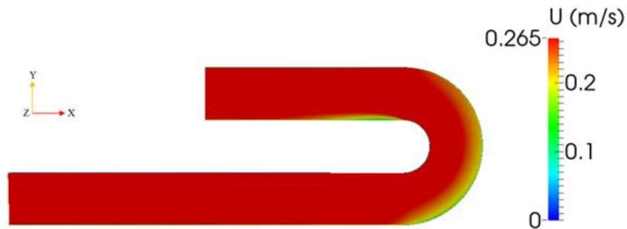
Figure 5.6: The distribution of water surface velocity (Standard k-\epsilon )
