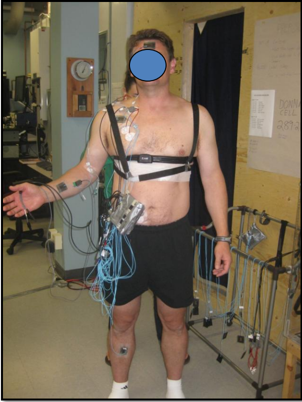
Figure 2.1. A participant fitted with heat flux and sEMG sensors.
