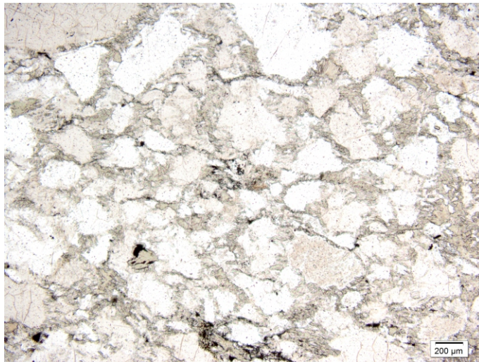
Figure C.4. Clean sandstone. Quartz and feldspar sand-size grains surrounded by fine mica, and quartz grains that result from the recrystallization, probably mainly by subgrain rotation. Left photo, plane-polarized light. Right photo, same view under crossed polars.
