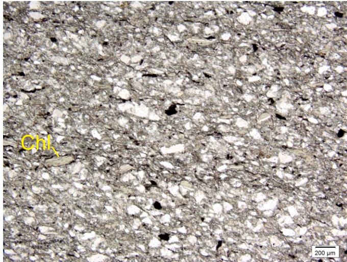
Figure C.3. Poorly-sorted matrix-rich sandstone. Silt- and sand-size quartz grains and porphyroblasts of chlorite embedded in a recrystallized matrix containing muscovite, and chlorite. Left photo, plane-polarized light. Right photo, same view under crossed polars.
