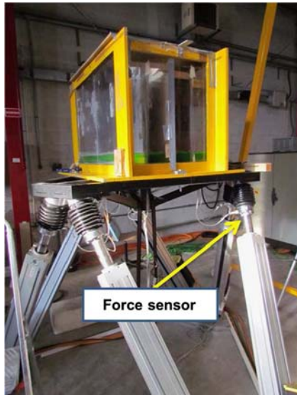
Figure 2.11: The tank mounted on Mistral Hexapod
