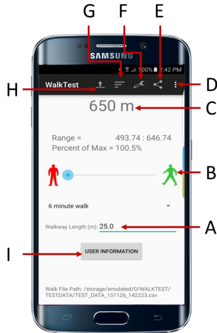
Figure 10 TOHRC Walk Test application. (A) Walkway length; (B) Start trial, (C) Distance walked; (D) About, Help; (E) Share output; (F) Settings; (G) Results tables; (H) Load previous data; (I) Enter patient demographics.
