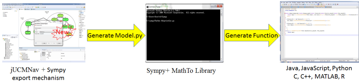
Figure 5.2: Overview of the transformation from goal/feature models to SymPy and then to executable functions
