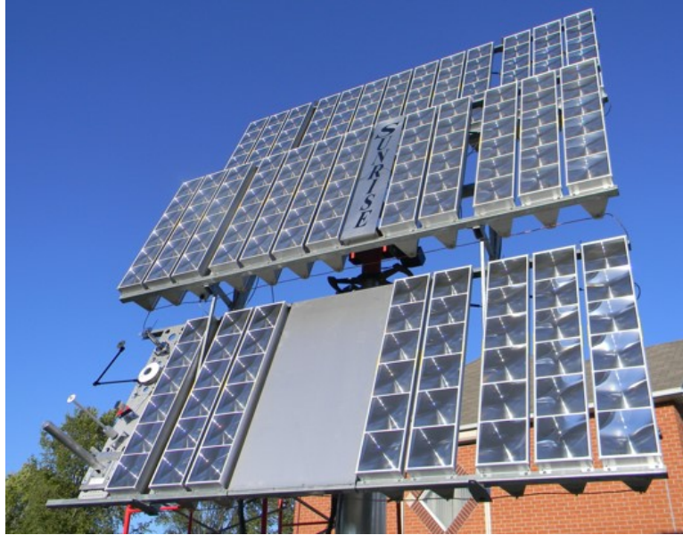
Figure 1.6: An installed CPV system at our solar test site at the University of Ottawa.
