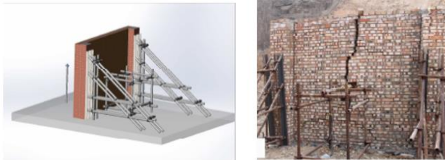
Figure 2-21. Test setup and result of wall retrofit with one side of polyurea (Wang et al., 2016)
