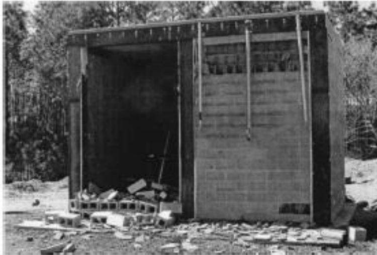
Figure 2-25. Comparison of control and retrofit wall for Test 1. (Davidson et al., 2004)
