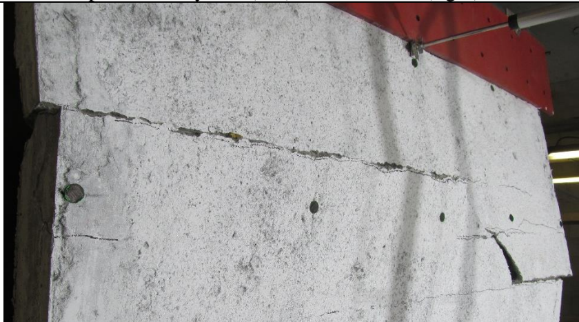
Figure 5-28. Polyurea and Shotcrete Retrofit Comparison (Polyurea from Ciornei, 2012)
