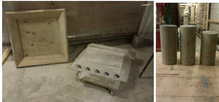
Figure 3-20. The shotcrete panel is cored for the cylinders. The smaller core represents the size for the first set of shotcrete cores
