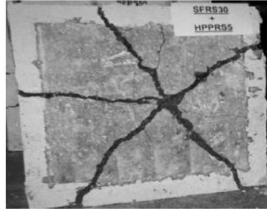
Figure 2-34. Test setup and results of the panel with a mixture of fibers (Cengiz et al., 2004)
