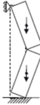
Figure 2-7. Beam Bending Failure (Sharif et al., 2007)
