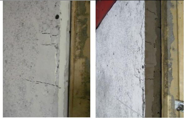
D) Main Crack Widening at Shot 5 (left) and Shot 6 (right)
