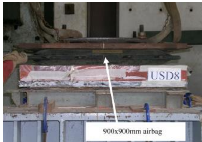
Figure 2-36. UDL testing setup (Maalej et al. 2010)
