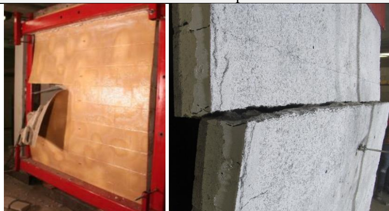
Figure 5-27. Polyurea Retrofit Comparison (Polyurea photos from Ciornei, 2012)
