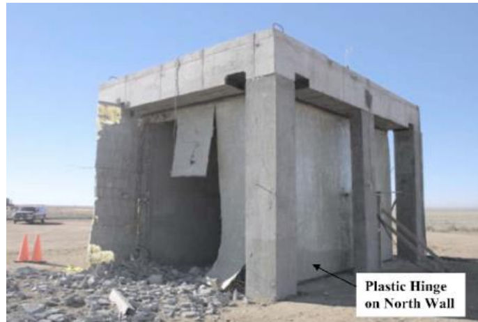
Figure 2-43. Results of the test. The north and south walls remained intact. (Maji et al., 2008)
