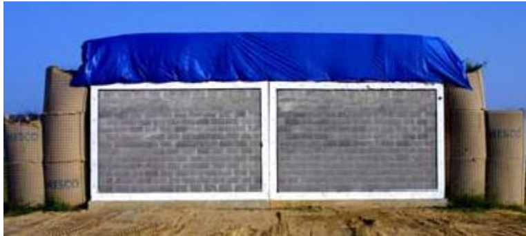
Figure 2-26. Setup of Wall 1 explosive test. (Johnson et al., 2004)
