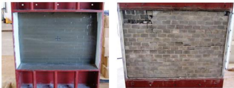
Figure 2-23. Wall 3 retrofit with polyurea and POSS. (Irshidat et al., 2011)
