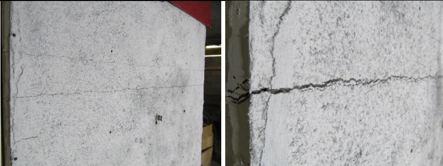
D) Main Crack Widening at Shot 5 (left) and Shot 6 (right)
