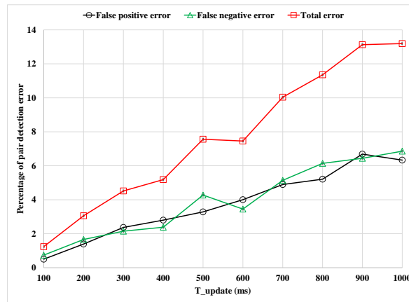
Figure 6.9: Percentage of pair detection error for different T_{update} values, B = 500bytes , T_{D2D} = 100ms
