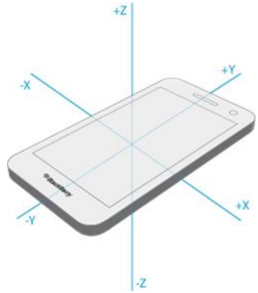
Figure 29: BlackBerry Z10 accelerometer components.
