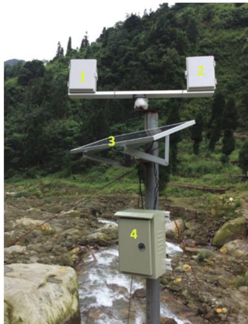
Figure 6: Stereo Imaging Configuration on the Longxi River where 1 and 2 are the cameras used, 3 is the solar panel used to power the system and 4 is a box where additional equipment is stored (W. Li et al., 2019)
