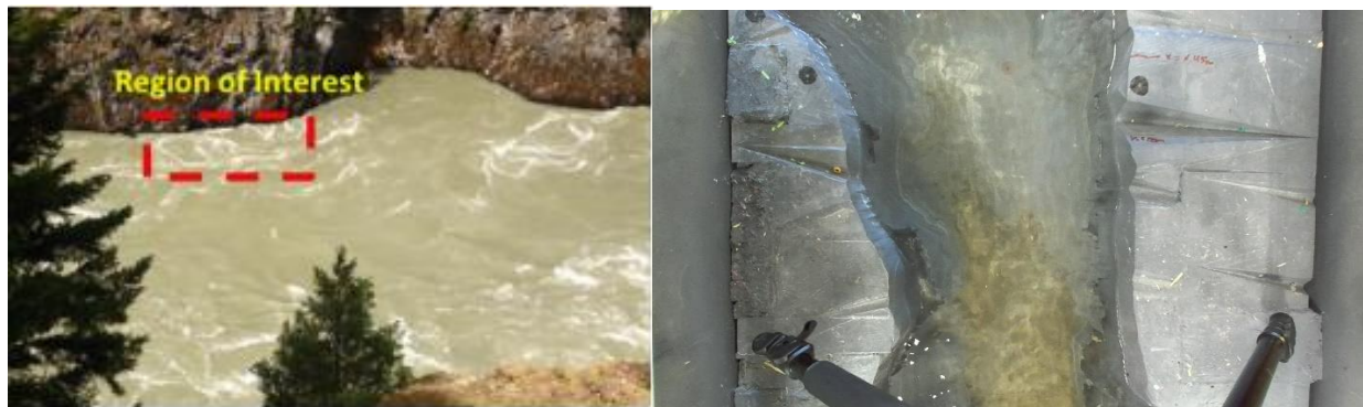
Figure 25: Left) Region of Interest (ROI) in the Black Canyon (Ansari et al., 2018) Right) NADIR view of ROI in lab model
