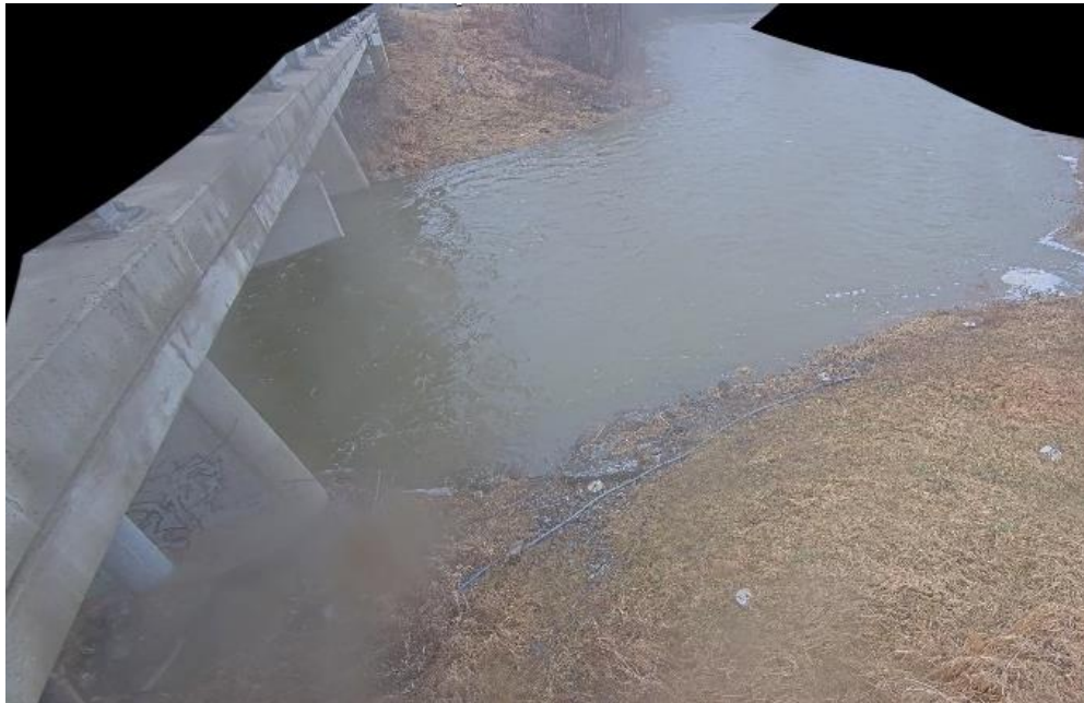
Figure 66: Top) Left bank vs right bank camera vector plot zoomed in towards left bank. Bottom) Frame from left bank camera showing lack of surface texture along the left bank caused by glare
