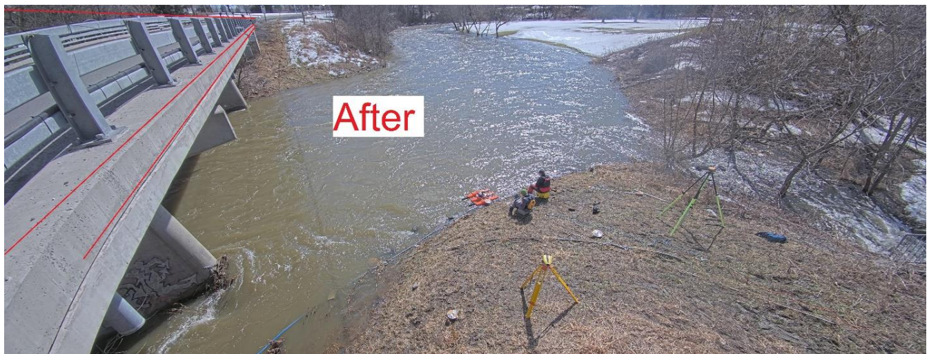
Figure 89: Distortion still affecting images post-distortion correction in the left bank camera
