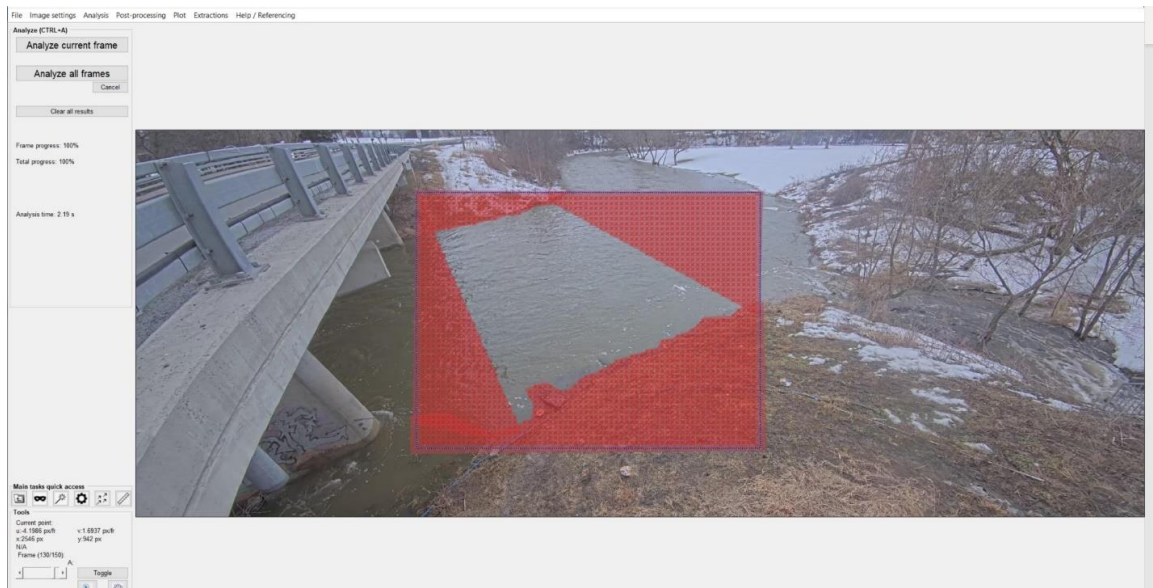
Figure 58: Example of Empty PIV vector field in PIVLab where the blue box represents the area being processed and the red indicates areas that have been masked out
