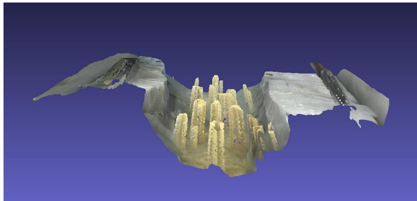
Figure 98: Reconstructed 3D Point Cloud of the Canyon Model created with the Stereolabs ZED2i Camera displaying how tracer particles are stretched from the water surface to the canyon bed
