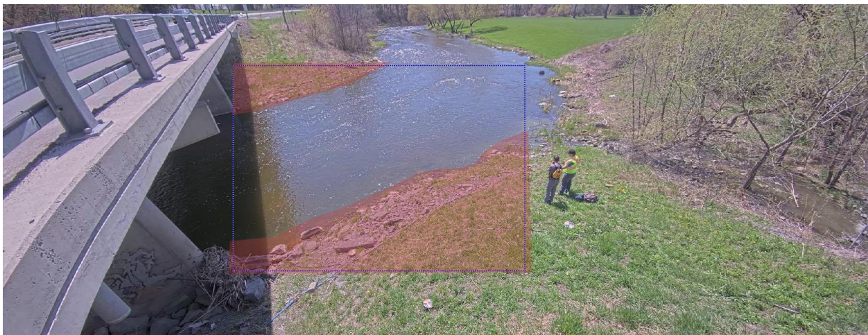
Figure 36: User-defined region of interest with masked banks for a left bank video at the Castor River
