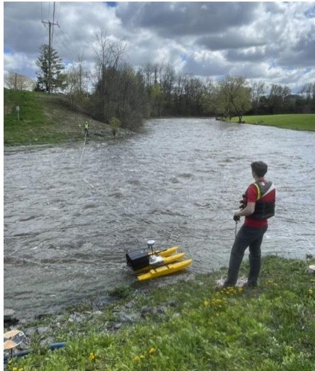
Figure 23: Author and supervisors performing an ADCP zig zag survey from May 5th, 2023
