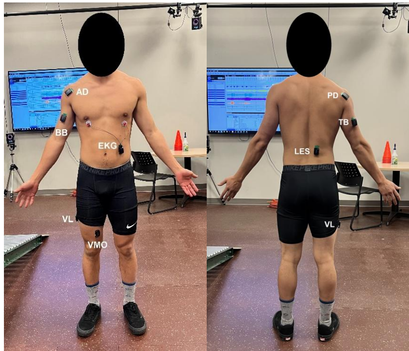
Fig. 6.1. The anterior (left) and posterior (right) perspectives of the electromyography and electrocardiogram (EKG) sensor setup. AD = anterior deltoid; BB = biceps brachii; VL = vastus lateralis; VMO = vastus medialis obliquus; PD = posterior deltoid; TB = triceps brachii; LES = lumbar erector spinae. Note that there was only one VL sensor despite being depicted in both perspectives.
