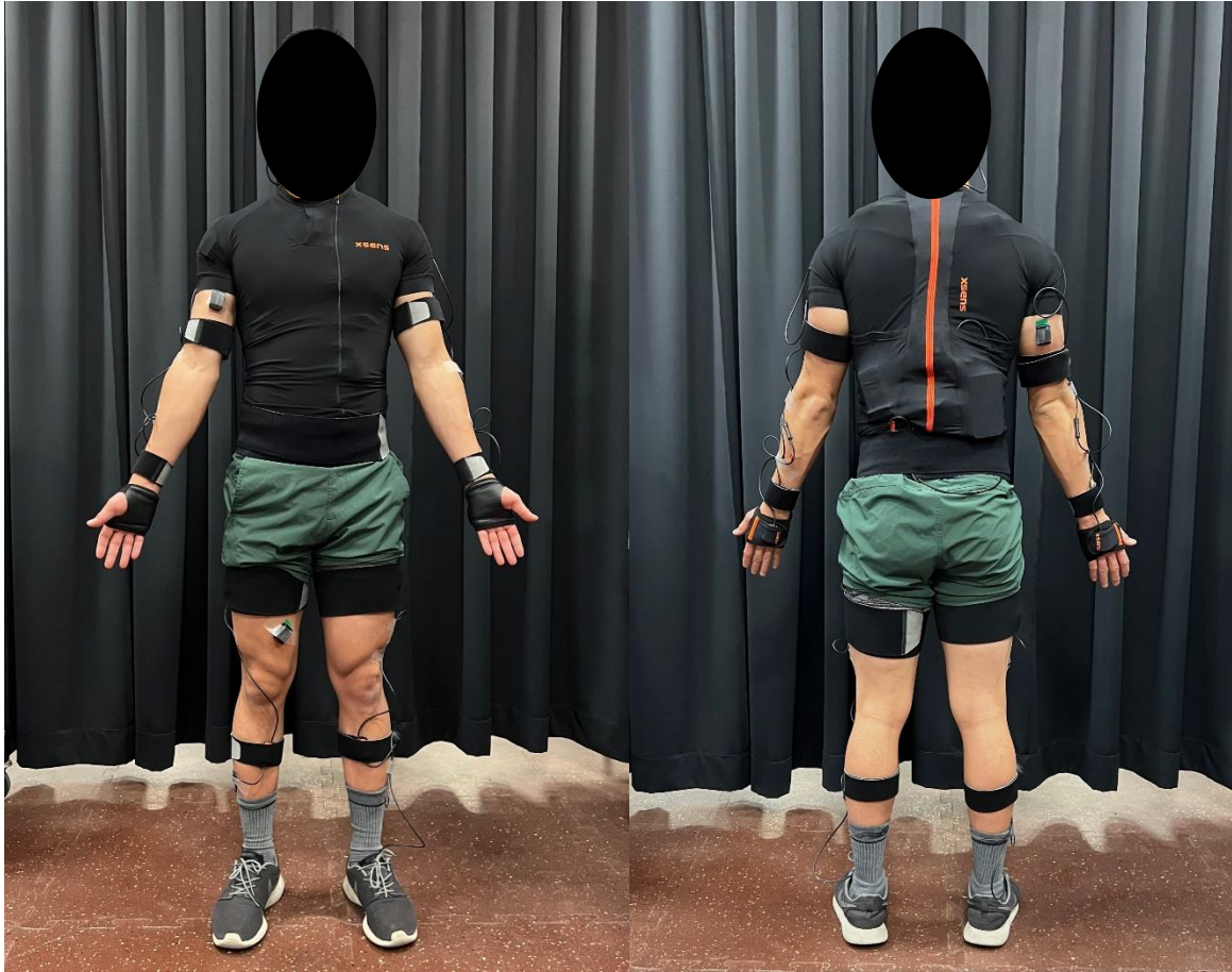
Fig. 6.2. The Xsens inertial motion capture suit with 17 inertial measurement units: one each on the head, sternum, and pelvis; and bilaterally on the shoulders, upper arms, forearms, hands, thighs, shanks, and feet.
