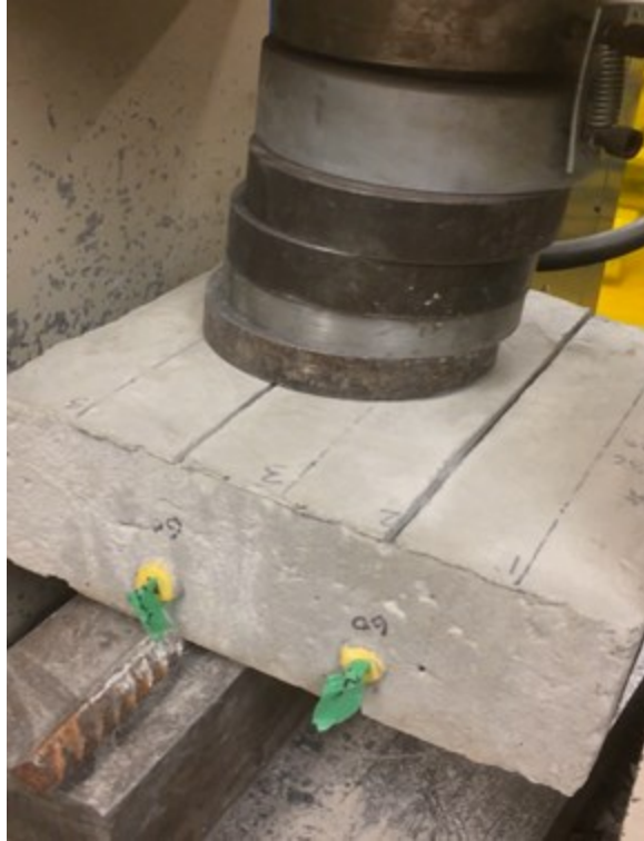
Figure 3.12: Modified Split Cylinder Test for Laboratory Rebar Removal
