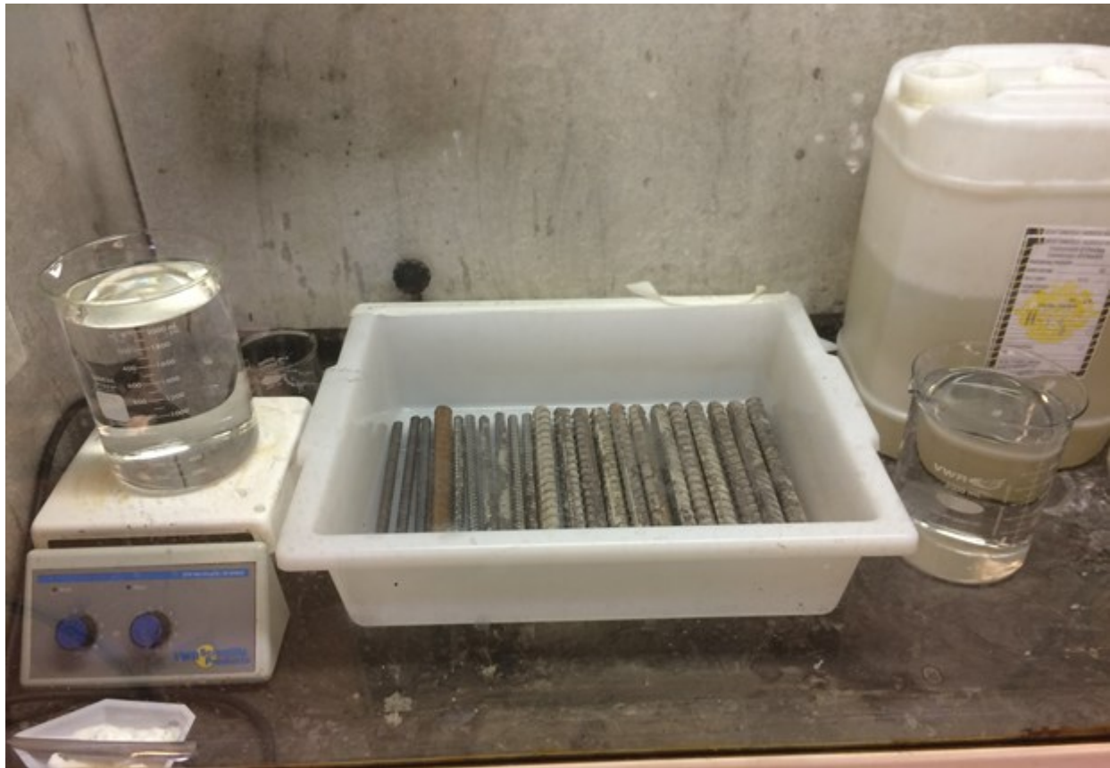
Figure 3.14: Gravimetric Mass Loss Testing according to ASTM G1-03.
