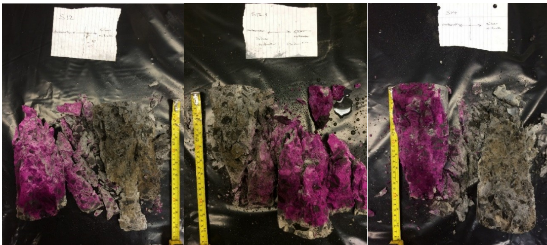
Figure 3.26: Split Cylinders Tested for Carbonation Front (left) and Chloride Penetration Depth (right)
