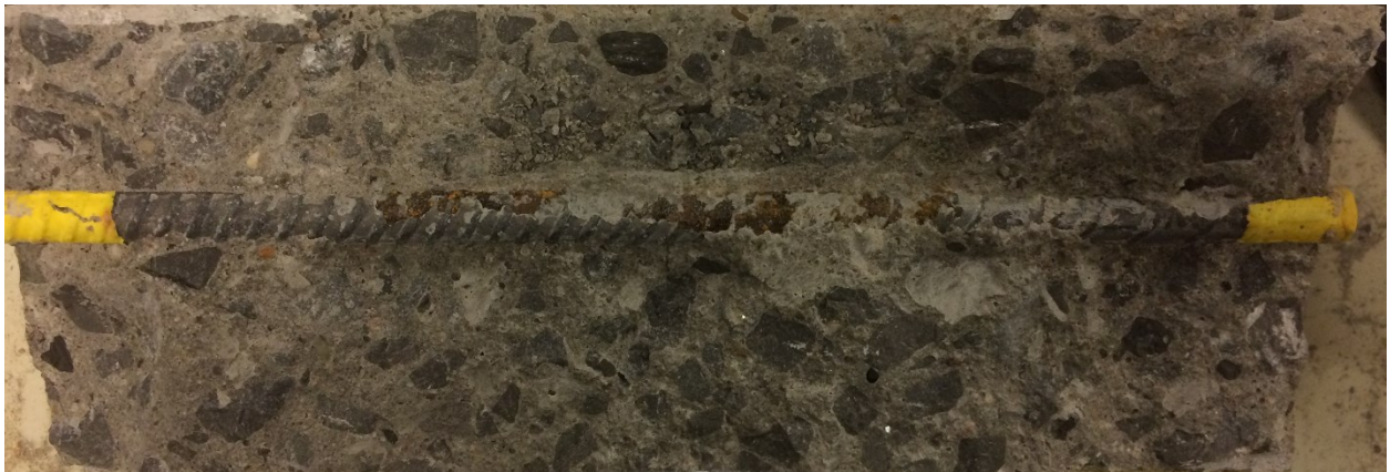
Figure 3.13: Laboratory Rebars Within Split Concrete
