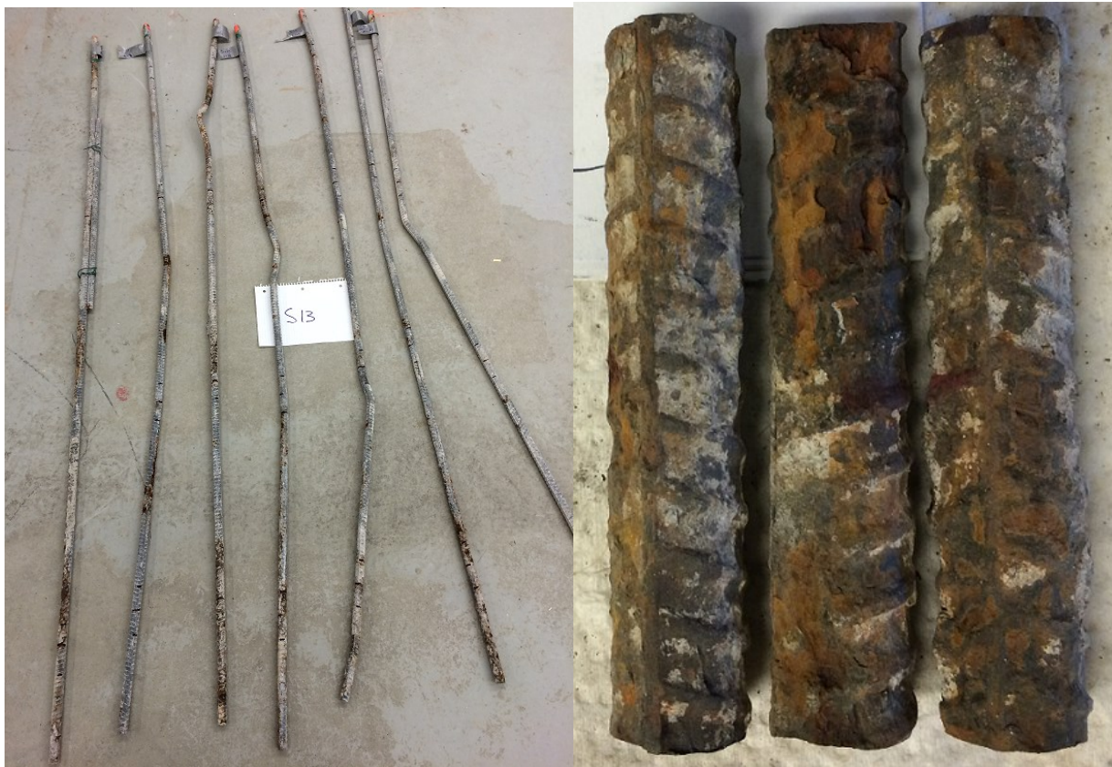
Figure 3.28: North Channel Bridge Reinforcement Specimens
