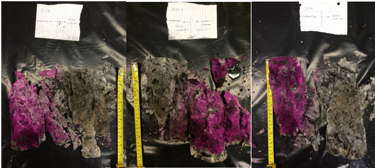
Figure 4.48: Split Cylinders Tested for Carbonation (left) and Chloride Penetration Depth (right)
