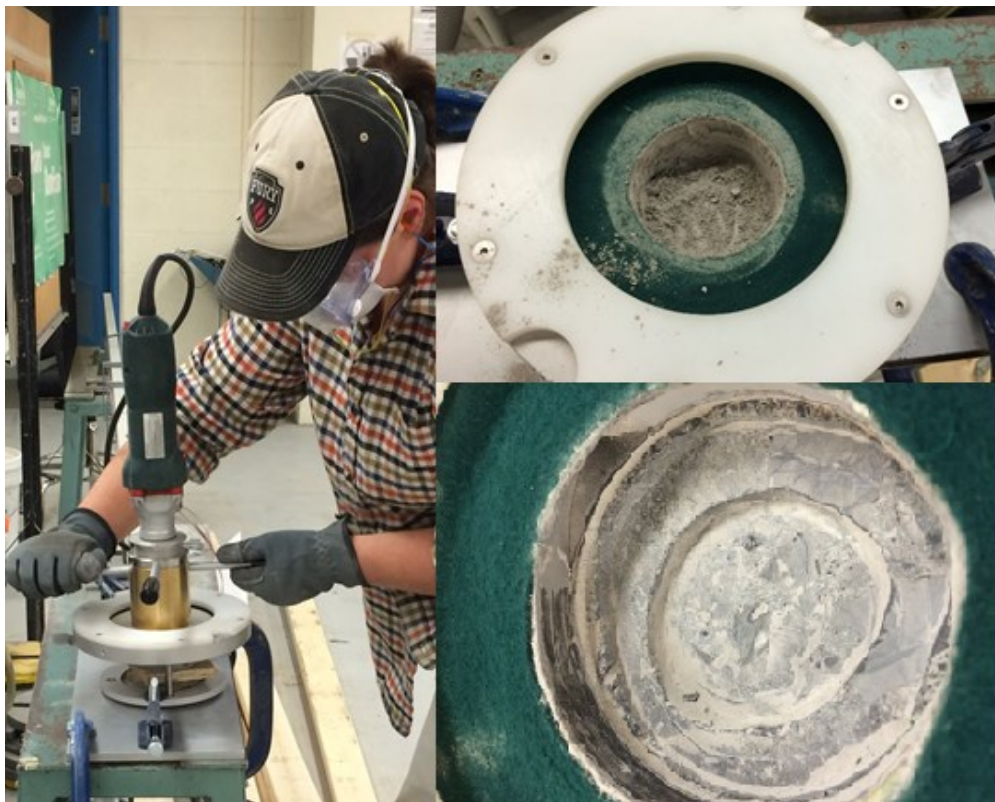
Figure 3.27: Profile Grinding Process
