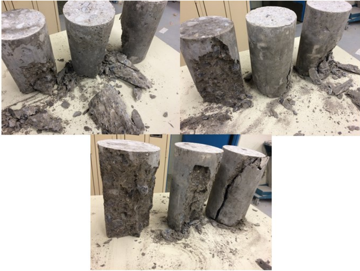
Figure C.0.2: Mix #1-28 Day Rupture Cylinder Failure
