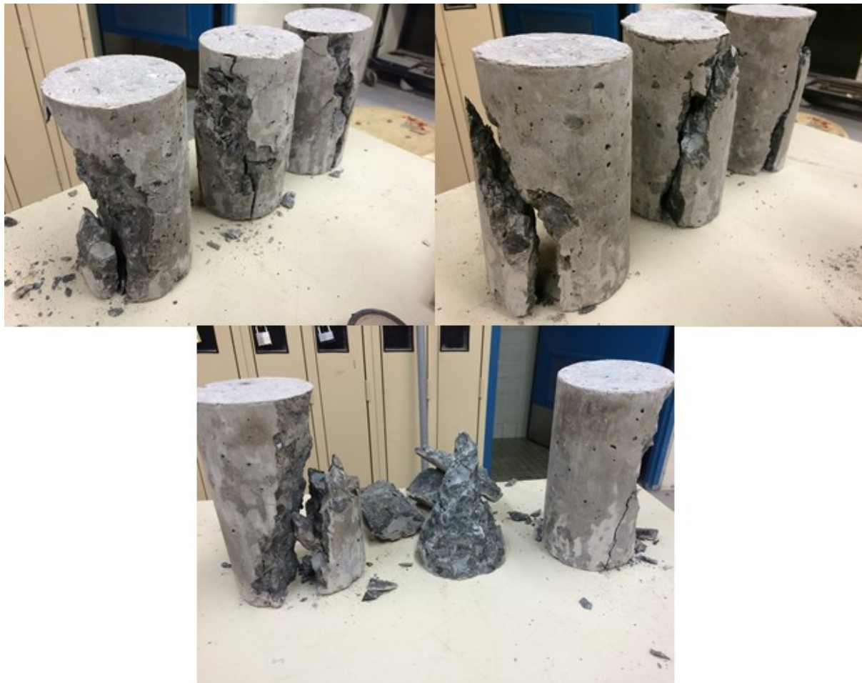
Figure C.0.1: Mix #2-28 Day Compression Cylinder Failure
