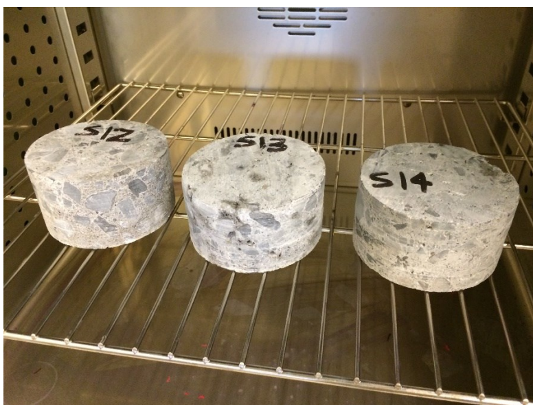
Figure 3.25: Specimens for ASTM 642 Testing
