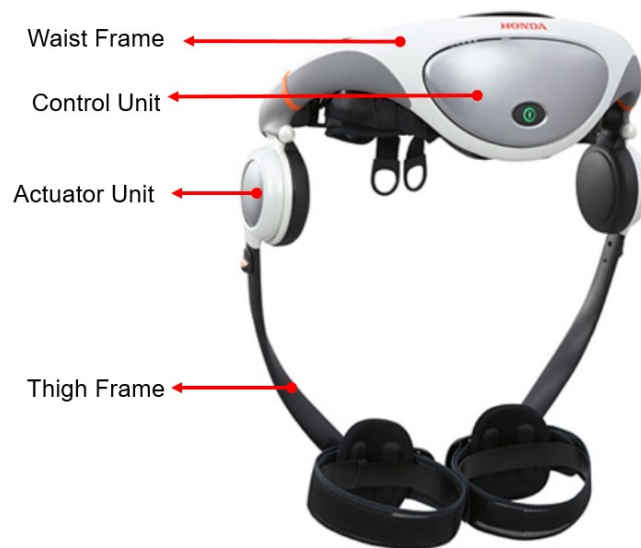
Figure 2-12: Honda Stride Management Assist with description of components [53].
