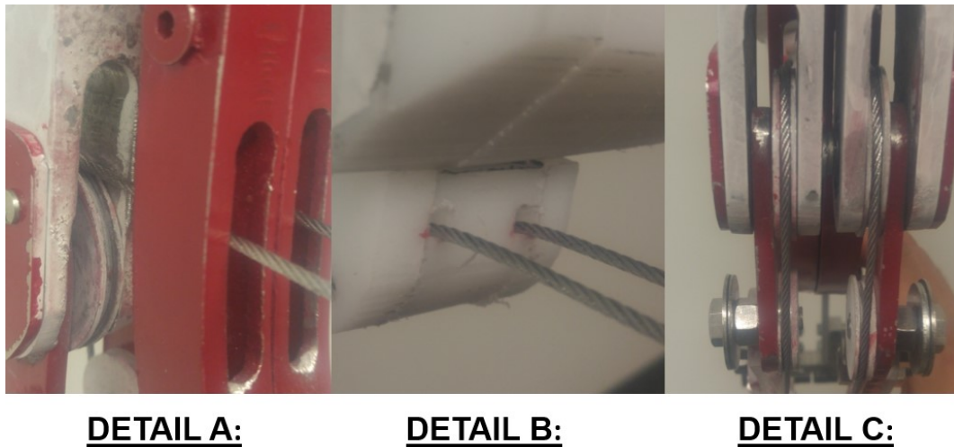
Figure 5-8: Photographs of three zones of friction. Friction at back slot (detail A), friction on SU (detail B) and friction on pulleys (detail C).
