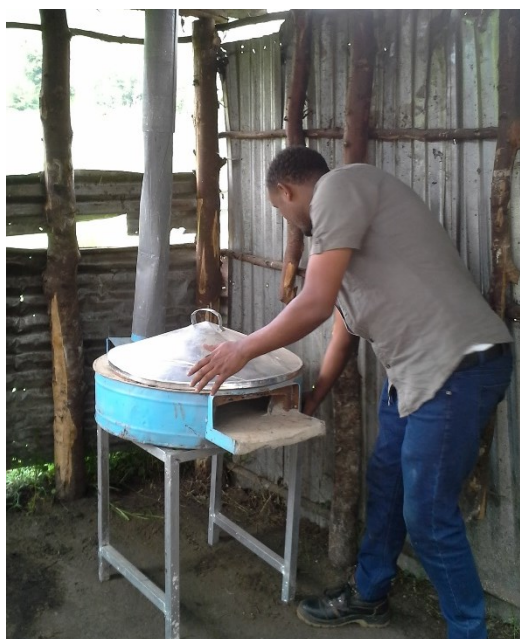
Study coordinator helping the Lilu Omoti site set up the injera stove and ensuring that the chimney was correctly installed.
