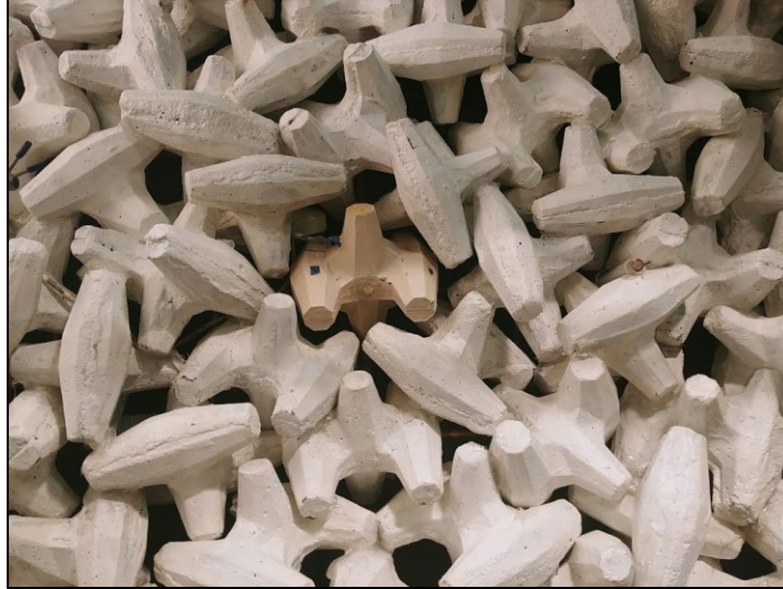
Figure 3-9. Typical setup of units in Core-Loc armour layer (instrumented unit at centre)
