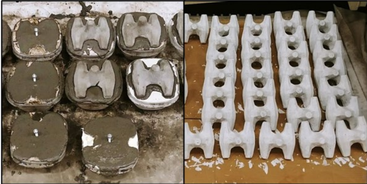
Figure 3-8. Model scale concrete armour unit manufacturing process (left). Finished, painted, custom concrete armour units (right).
