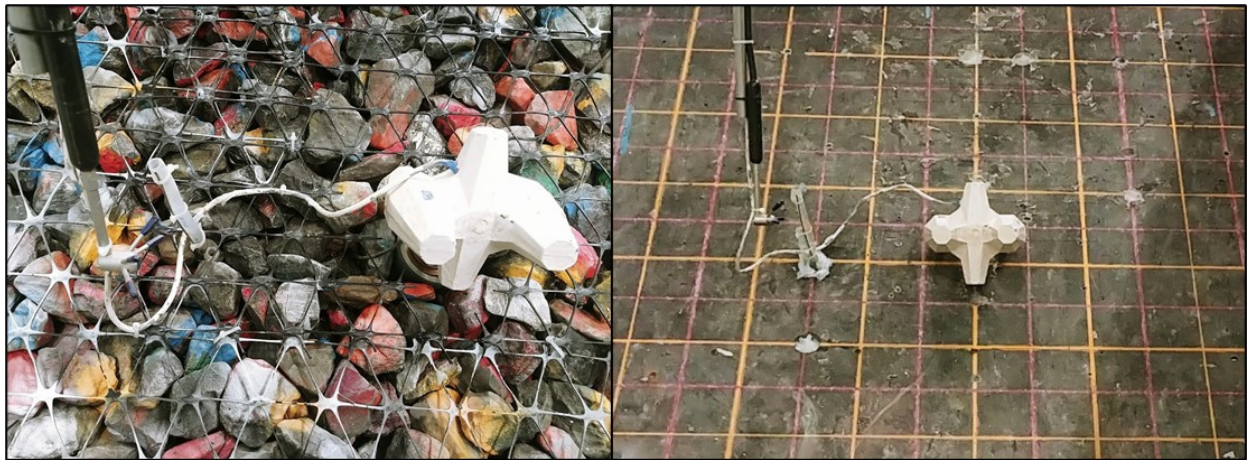
Figure 3-7: Top of filter layer, geogrid, and instrumented unit (left), Instrumentation wire, ADV connection, and pressure sensor apparatus mounted through PVC board (right)
