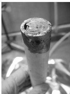
Figure 6.5 Picture of the excessive coking observed during operation of a button cell with the composition of Ni 0.7 Co 0.3 -YSZ at 850°C in pure biodiesel fuel.
