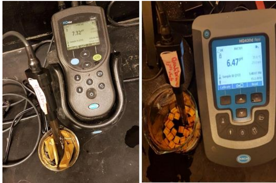
Figure 3.11: PH measuring with the Digital PH Meter
