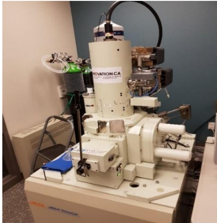
Figure 3.21: Scanning Electron Microscope (SEM), The Centre for Advanced Materials Research (CAMaR)
