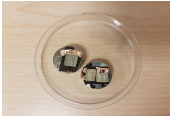
Figure 3.23: The prepared specimens for the SEM technique from Group A, and reference covered by gold as conductor
