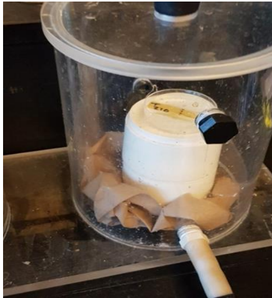
Figure 3.17: Pre-treated Impregnated sampled inside the vacuum
