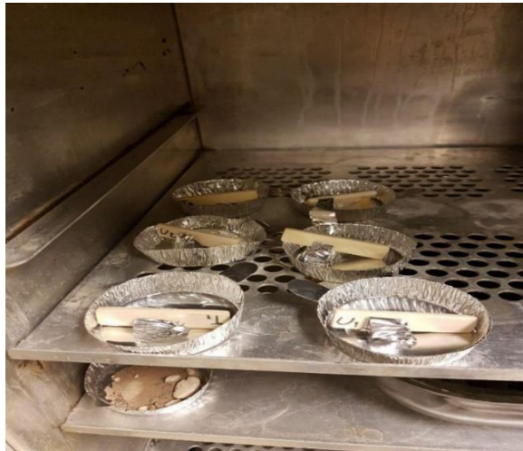
Figure 3.15: Drying process inside the oven
