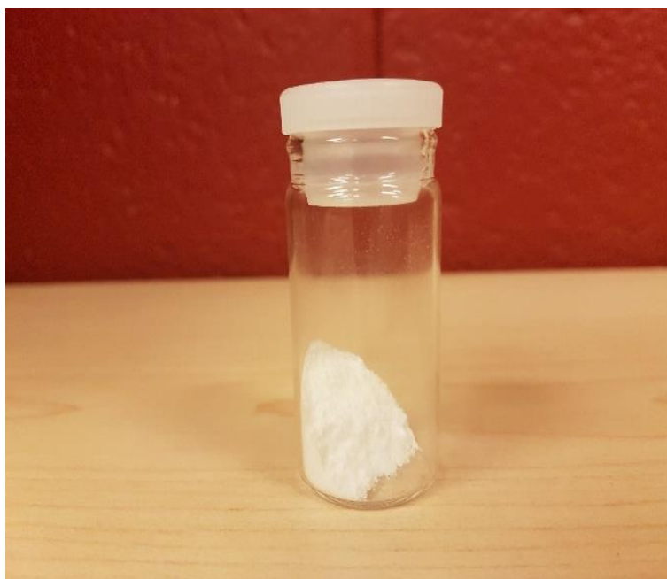
Figure 3.24: Silica nanoparticles extracted from the colloidal solution
