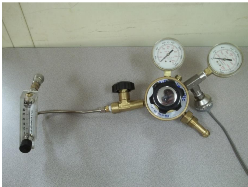
Figure 4.27 Gas pressure regulator and flow meter of the powder carrier gas
