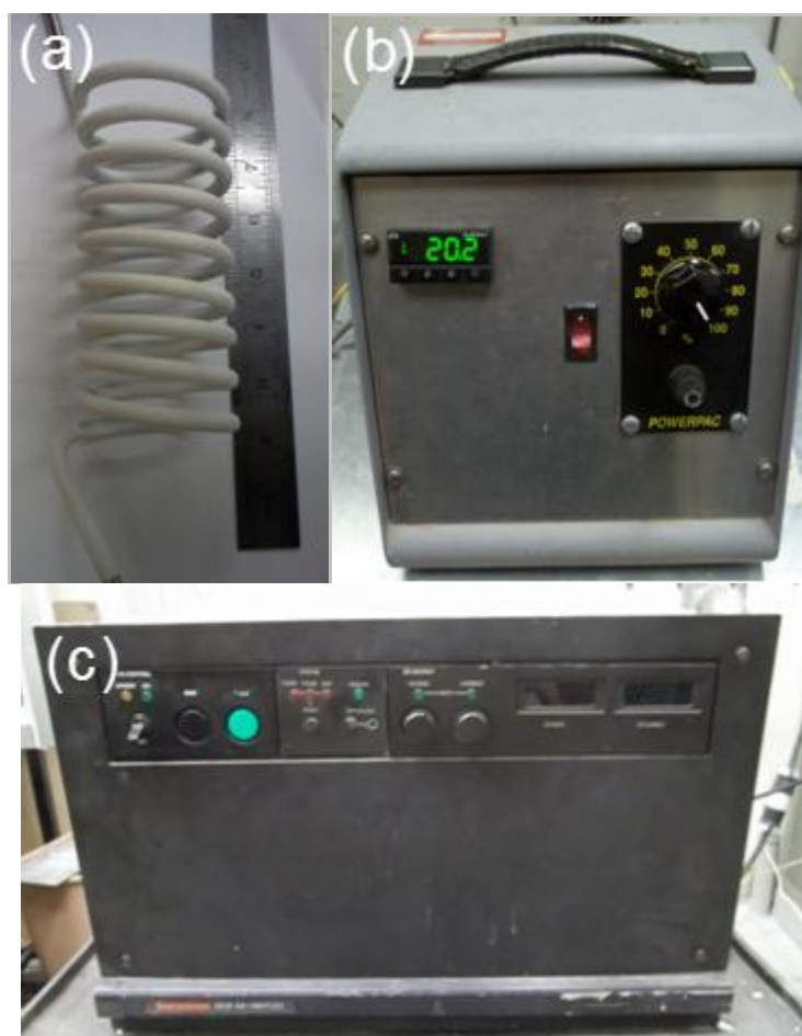
Figure 4.28 (a) Stainless steel powder heater coil alumina coated, (b) Temperature reader and (c) Power supply
