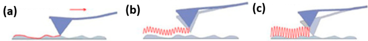
Figure 2.8: Operating modes of the tip in atomic force microscopy. (a) Contact mode , where the tip makes contact with the material surface and the repulsive force is detected. (b) Non-contact mode , where the tip is maintained a distance above the surface, and the attractive force is detected. (c) Tapping mode , where the tip is vibrated at a resonant frequency such that it contacts the material at the peak amplitude.
