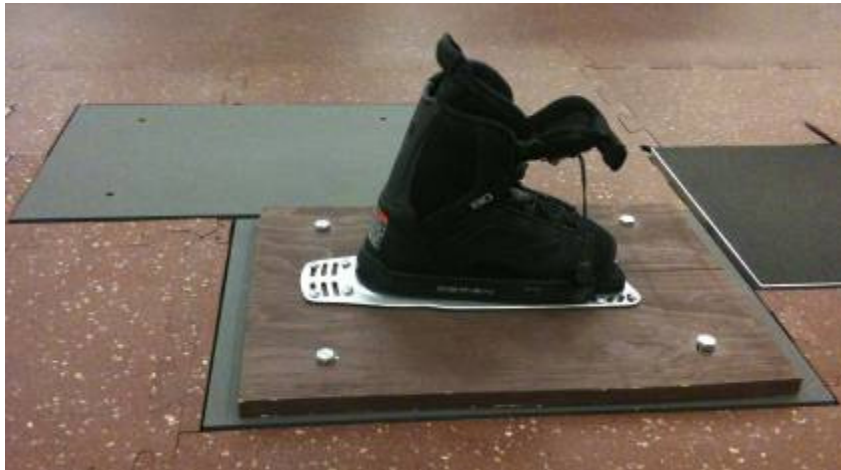
Figure 5: The test force platform (near) with the fixed water ski boot attached via a wooden top-plate and bolted with threaded holes. The support leg force platform (far) has no extra attachments and is situated adjacent and slightly posterior to the test force platform.
