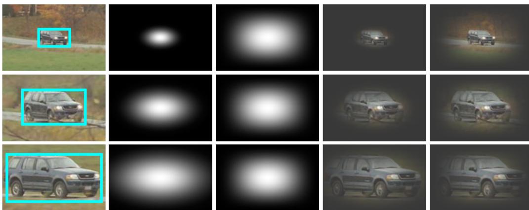
Figure 6.1: Gaussian and cosine window filtering raw pixel value example. The tracked region has a size of (175 \times 113) . First column: same regions with targets at three different scales (i.e., small (56 \times 32) , medium (110 \times 61) , large (164 \times 83) ). Second column: Gaussian windows according the target size (i.e., small (\sigma_w = .32, \sigma_h = .28) , medium (\sigma_w = .63, \sigma_h = .54) , large (\sigma_w = .94, \sigma_h = .73) ). Third column: cosine window for all the three examples (i.e, size (175 \times 113) ). Fourth and fifth columns: images filtered with Gaussian and cosine windows respectively. Figure shows how the fixed cosine window fails to represent the target compared to the Gaussian windows. The cosine window includes background for small targets and discards information for big targets.
