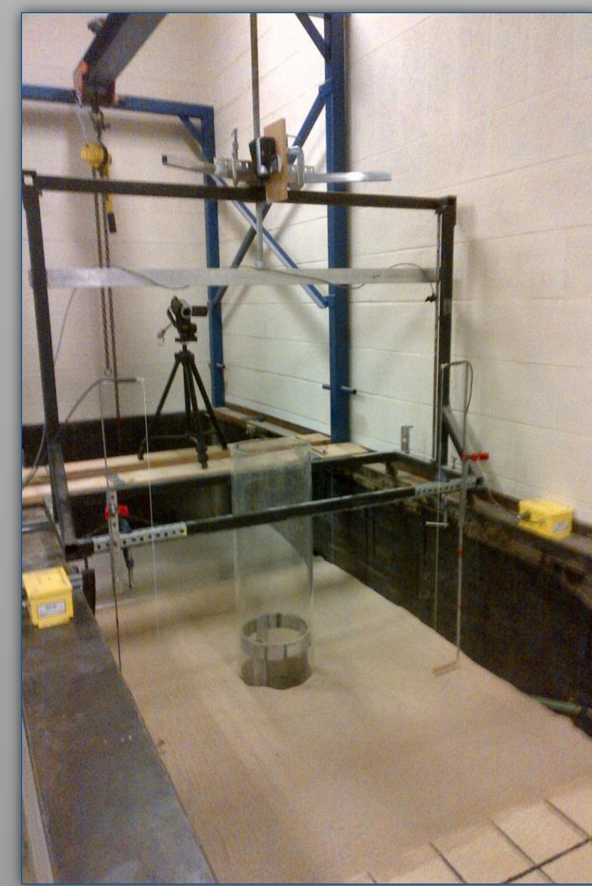
Figure 3: Plexiglas structure and sand bed set-up
