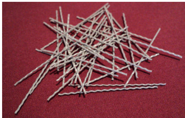
Figure 2.5: Example of crimped steel fibers
