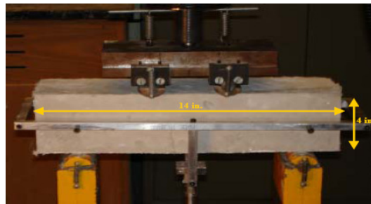
Figure 2.20: "Yoke" setup for measuring deflection [Adapted from Liao et al. (2006)]
