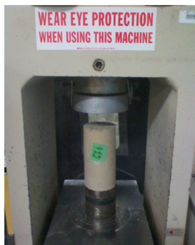
(a) Cylinder testing machine located at uOttawa Laboratory
