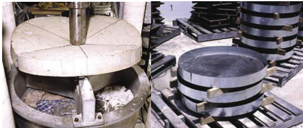
Figure 2.24: The round panel under test and the panel forms [Adapted from Bernard (2003)]
