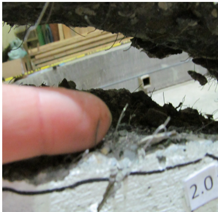
Figure 5.10: Pullout and straightening of hooked-end fibers after shear failure
