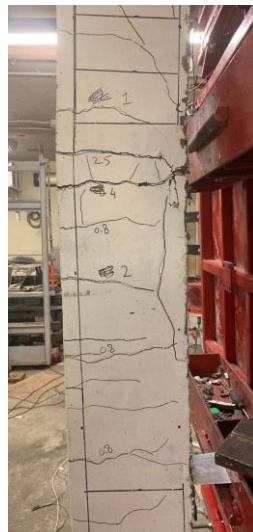
f) Concrete crushing at mid-span (Blast 2c)
