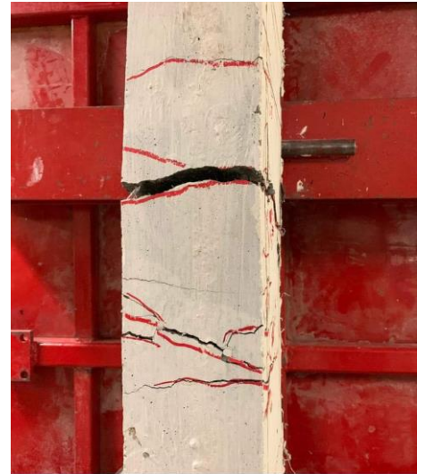
f) Mid-span fiber pullout (Blast 2c)
