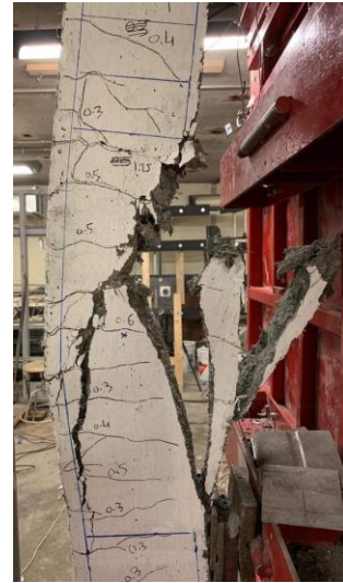
g) Mid-span concrete crushing (Blast 3b)
