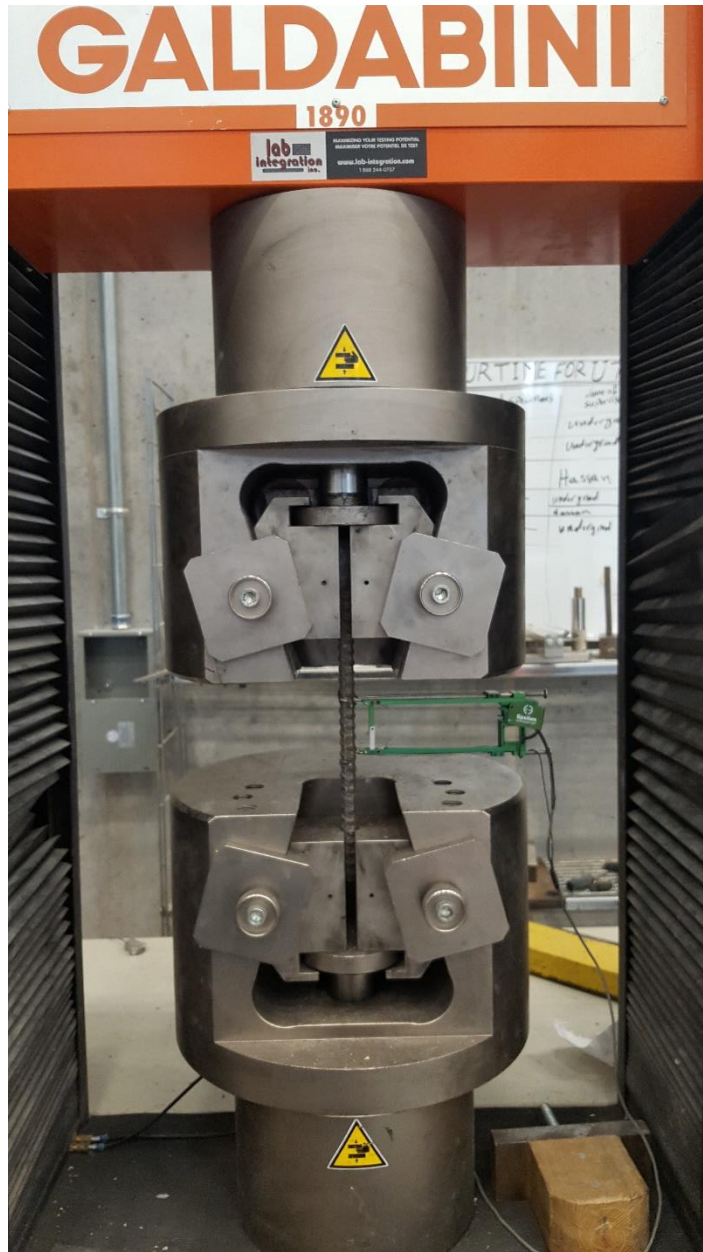
Figure 3-4 GALDABINI Universal Floor Standing Testing Machine; testing steel rebar
