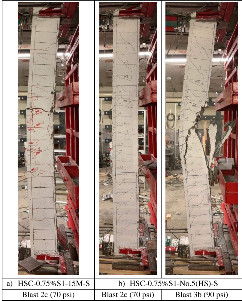
Figure 7-29 Photographs; effects of HSR in beams with synthetic fibers
