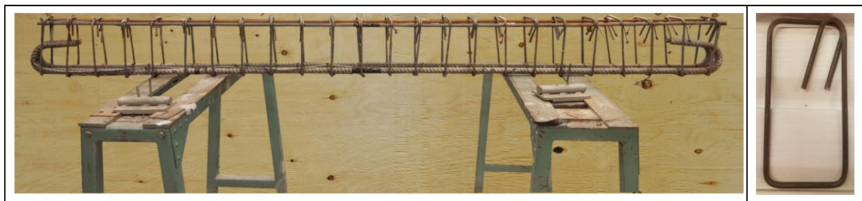
Figure 3-11 20M rebar with 10M compression bar and closed stirrups all the way
