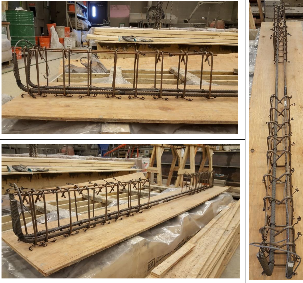
Figure 3-13 15M & No.5 rebars with stirrups
