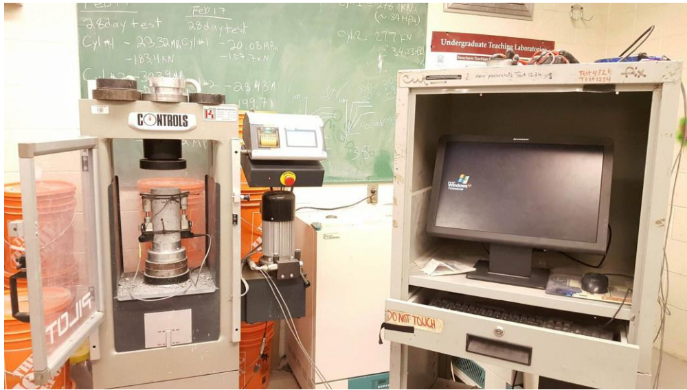
Figure 3-20 Cylinder testing setup
