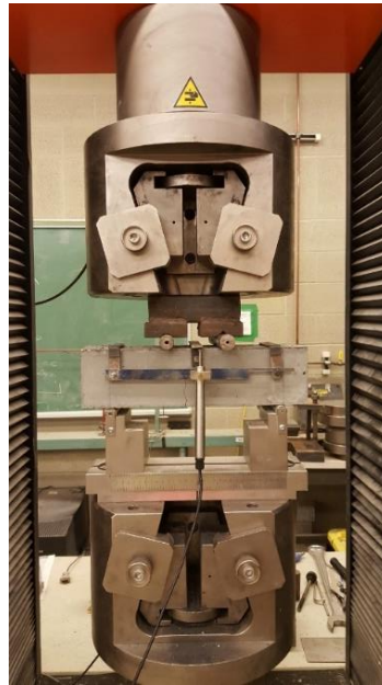
Figure 3-23 Flexural prism testing setup
