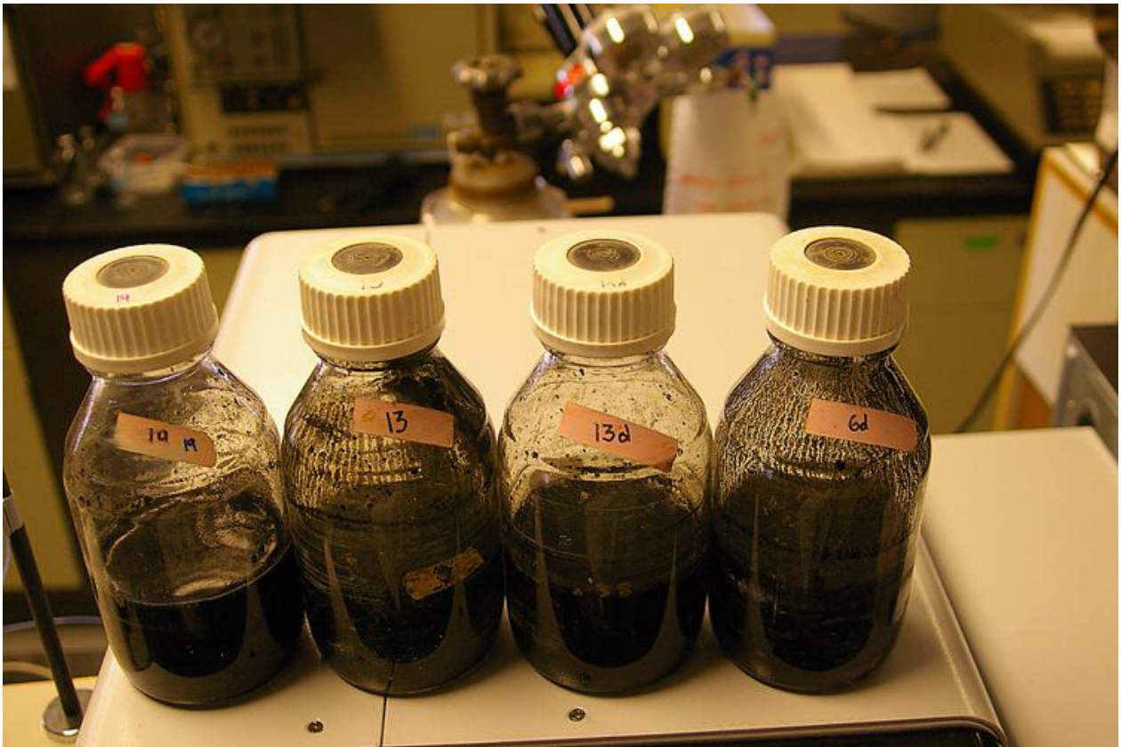
Figure A.6 - 500 mL bottles used for BMP tests.
