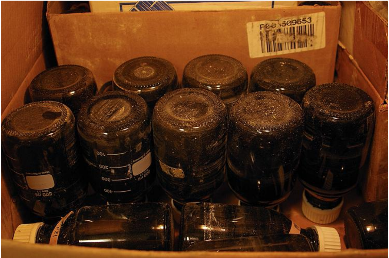
Figure A.8 - BMP bottles were incubated upside down to minimize biogas losses.
