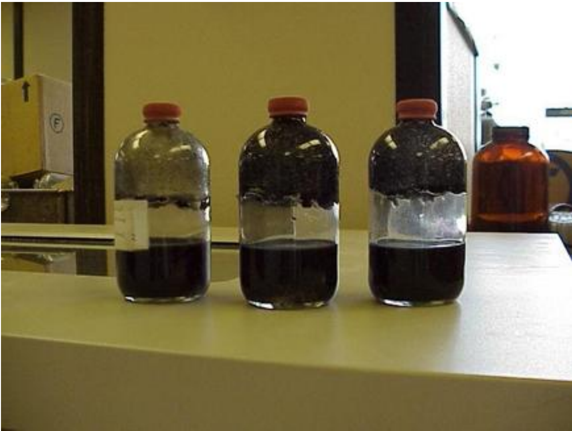
Figure A.7 - 125 mL serum bottles used for BMP tests.
