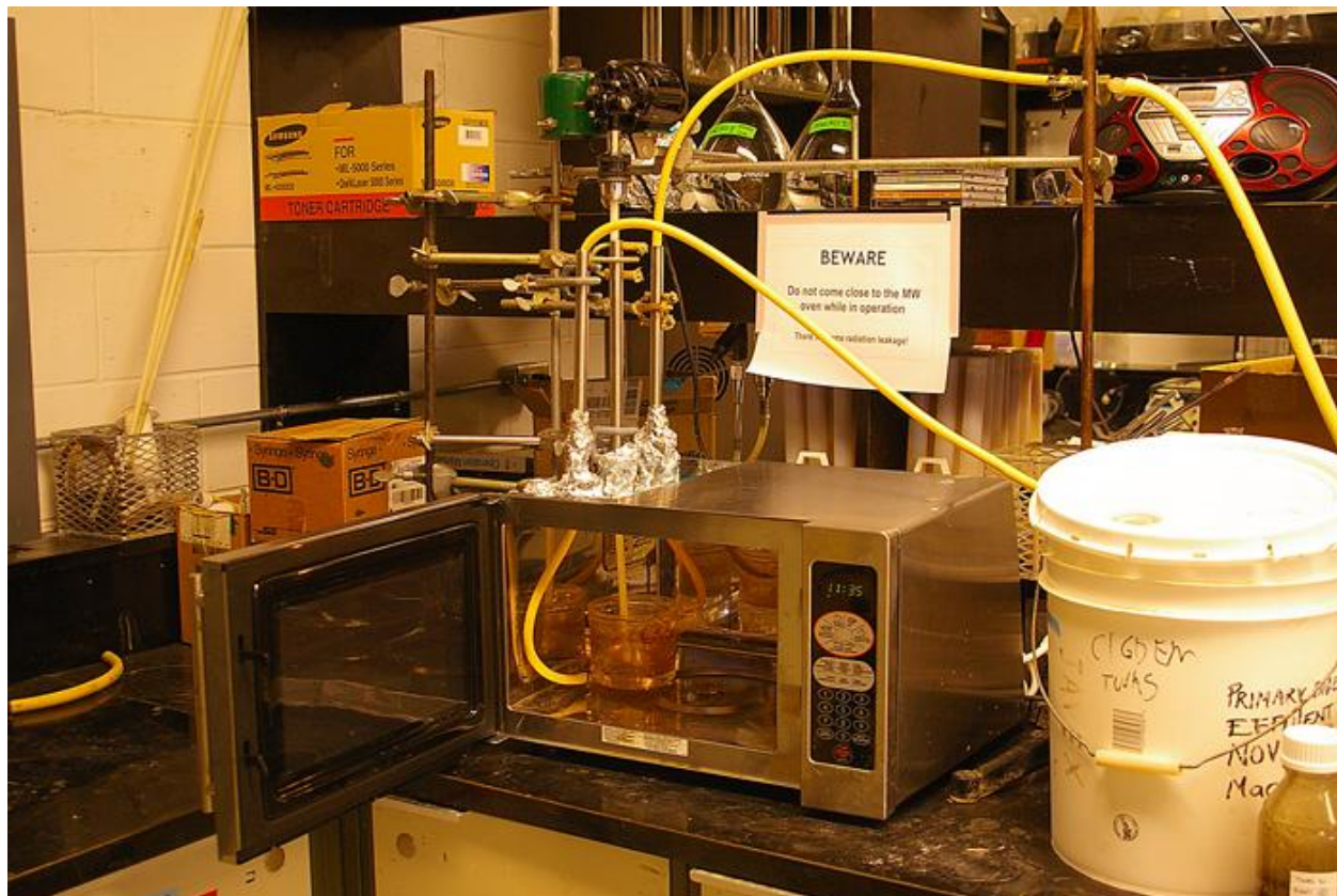
Figure A.1 - Athermal microwave radiation oven set-up.
