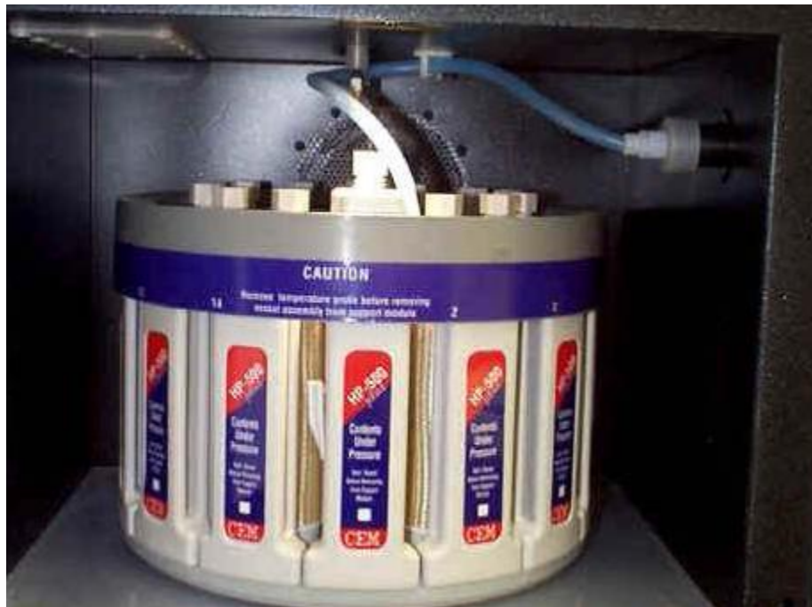
Figure A.5 - Vessel ready for pretreatment assembled in the rotating carousel with probes connected.
