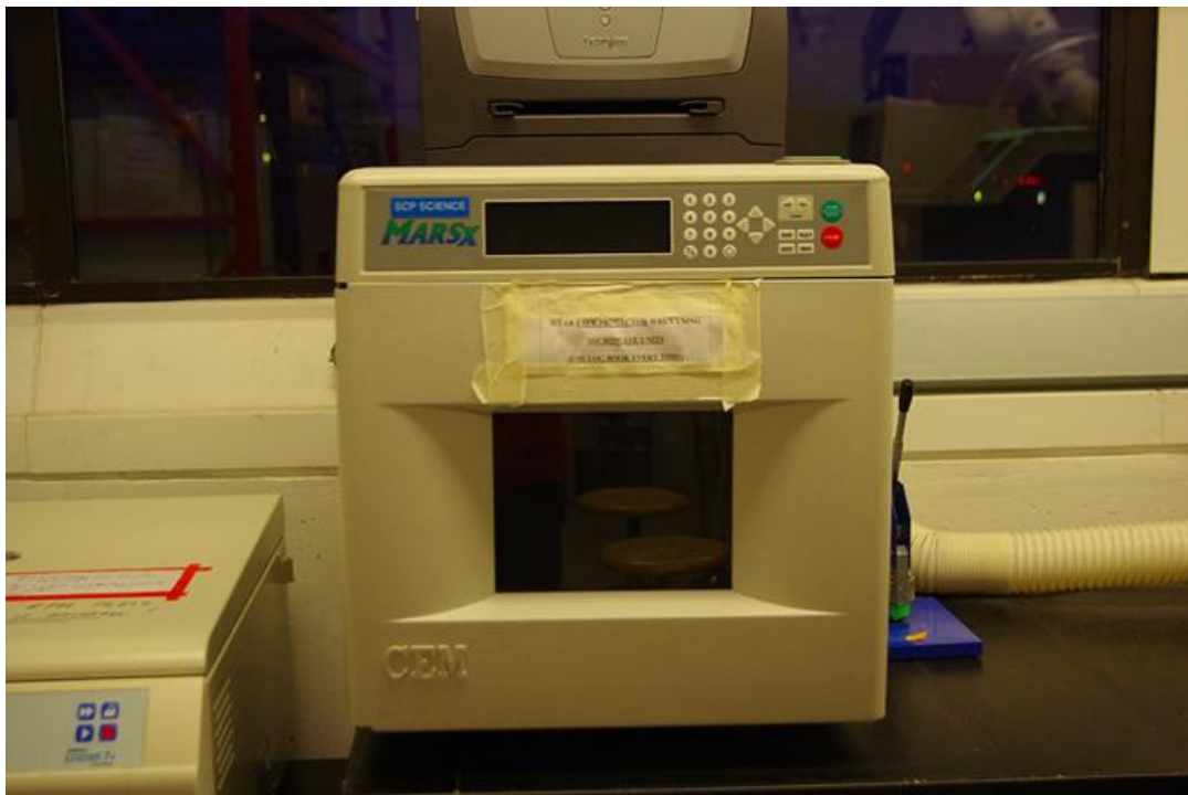
Figure A.3 - Microwave oven with pressure and temperature control
