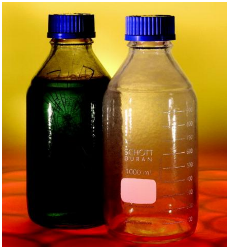
Figure A.9 - Schott borosilicate 1000 mL bottles used in the continuous reactors study.
