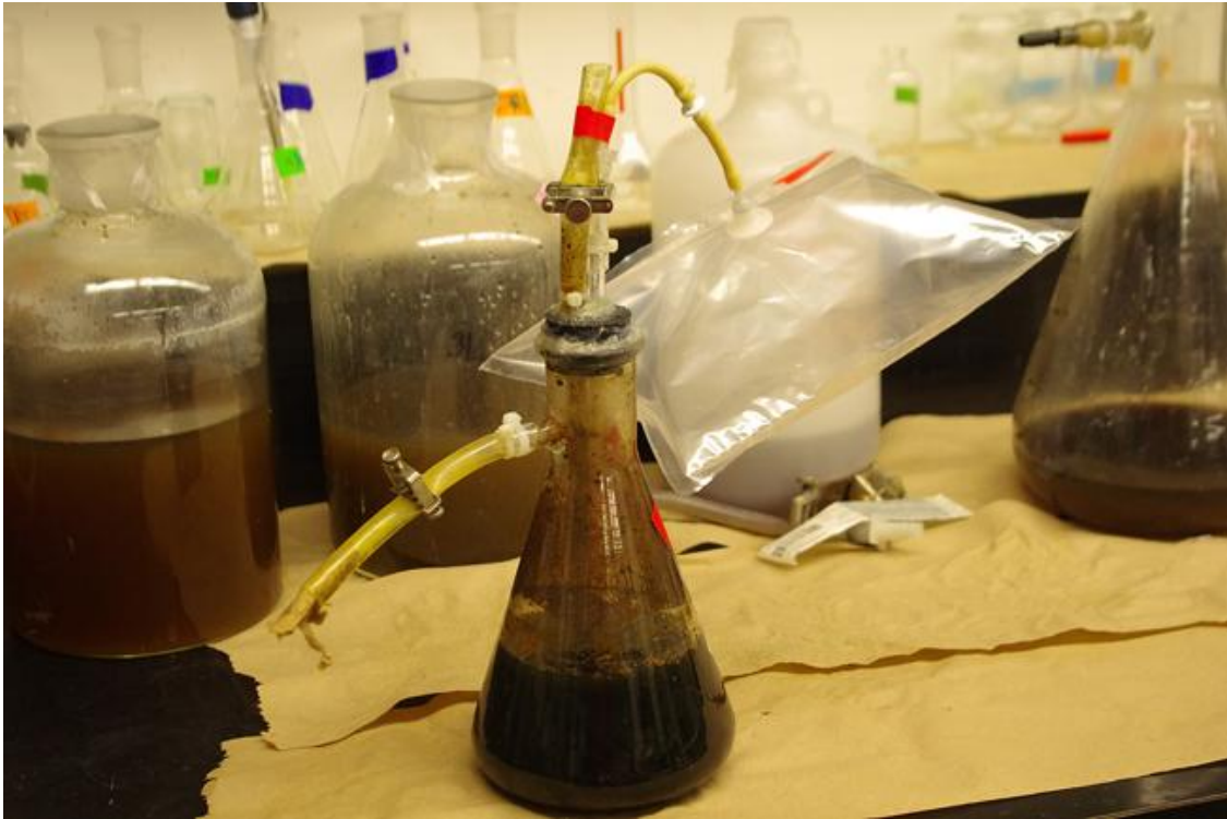
Figure A.10 - Erlenmeyer with the Tedlar gas bag system used to measure produced gas in the Chapter 6 work.
