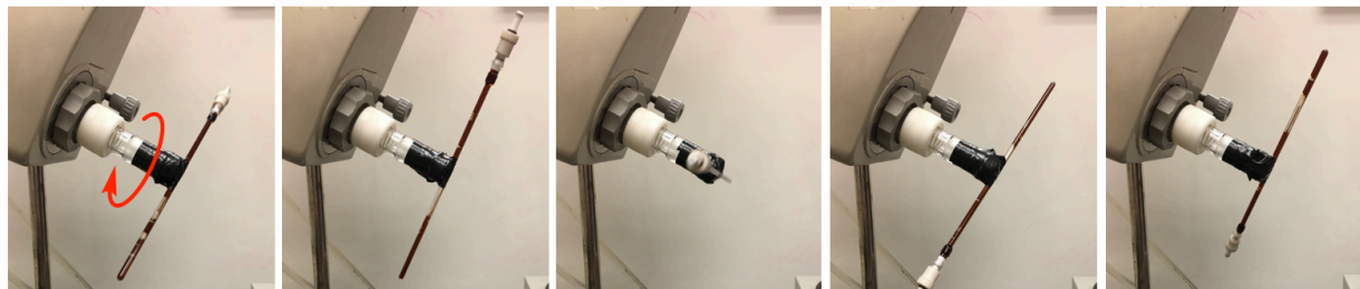
Figure 4.9. Time-lapse images showing setup for controlled mixing of filled NMR-tube reactions, using a J. Young NMR tube attached to the rotary evaporator with electrical tape. Efficient, controlled mixing is achieved by rotating at 15 rpm, a rate that enables an internal capillary tube to traverse the entire length of the NMR tube at every inversion.
