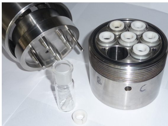
Figure 5.4. Photograph of the HEL7 Reactor, showing (left) temperature-controlled condenser tips, (right) glass-lined reactor wells sealed with white PTFE gaskets, and (center) an individual glass well liner.
