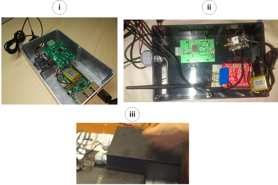
Figure 5.2: MVP gateway hardware box design: i) original metal box design; ii) plastic box hardware migration; iii) MVP's waterproof gateway box.
